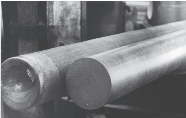
FIGURE 7.4 Surface appearance of 285-mm DC-cast billets from AA7055 alloys: (left) without ultrasonic melt processing and (right) with ultrasonic melt processing.
