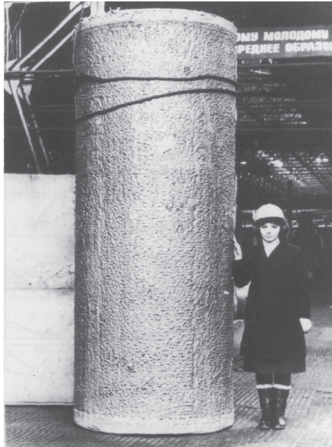
FIGURE 7.9 One of the largest ingots (1200-mm diameter, 10-ton weight) from an AA2324 alloy with nondendritic structure obtained by casting with ultrasonic melt processing in the billet sump.
