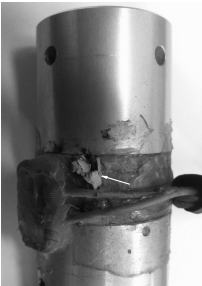
FIGURE 13.2 A piezoceramic element fractured due to overloading (arrow points at fractured fragments).
