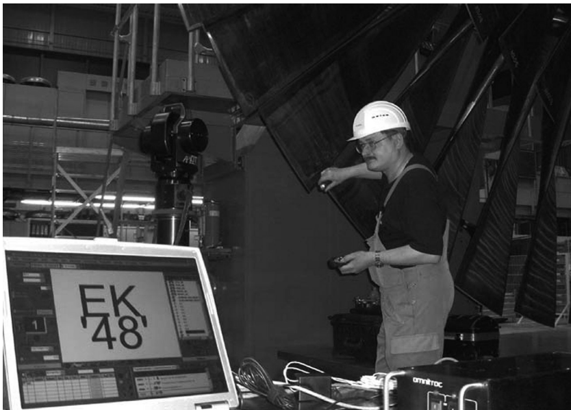
FIGURE 3.49 Power generation turbine blade inspection. (Courtesy of Automated Precision, Inc., Rockville, MD.)
