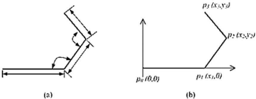
**FIGURE 3.10** Dimensioning the control polygon of a planar cubic Bézier curve. (a) Segment lengths and included angles are dimensioned. (b) Coordinate dimensioning of the control points.
