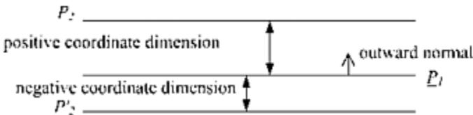
**FIGURE 5.16** Dimensioning the relative position of a nonoriented plane and an oriented plane when they are parallel.
