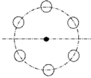
**FIGURE 7.11** A symmetric pattern of six holes. When translationally swept perpendicular to the plane that contains them, we get a 6-tuple of parallel cylinders that belongs to the prismatic class.
