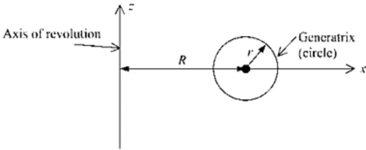
**FIGURE 4.8** A dimensioning scheme for the torus, viewed as a surface of revolution. For a ring torus  $R > r$ , for a horn torus  $R = r$ , and for a spindle torus  $R < r$ .
