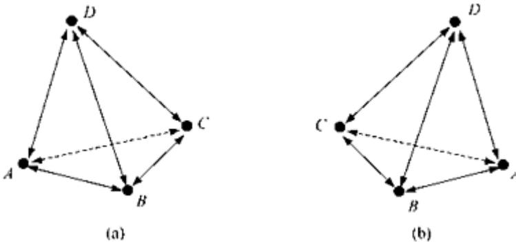
**FIGURE 9.3** Dimensioning a solid tetrahedron by specifying its six edges. (a) and (b) are mirror reflections of each other.
