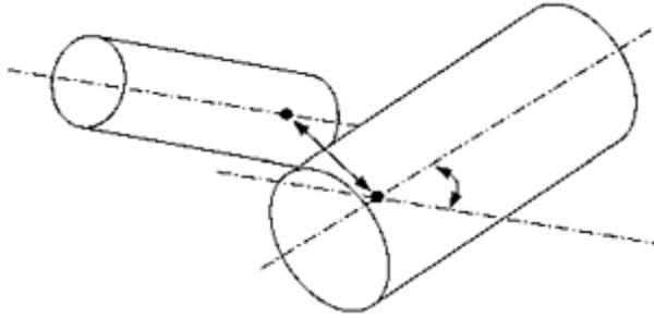
**FIGURE 7.4** Dimensioning the relative position of two cylinders whose axes are skew. The twist angle may be given as a positive or negative dimension to indicate chirality.
