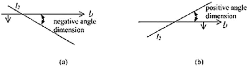
**FIGURE 5.11** Dimensioning the relative position of an oriented line  $l_1$  and a nonoriented line  $l_2$ , when they intersect at a point. The smaller angle between the two lines, ignoring the orientation of  $l_1$ , is dimensioned. (a) A clockwise rotation from the oriented line to the nonoriented line leads to the negative dimension. (b) A counterclockwise rotation from the oriented line to the nonoriented line leads to the positive dimension.
