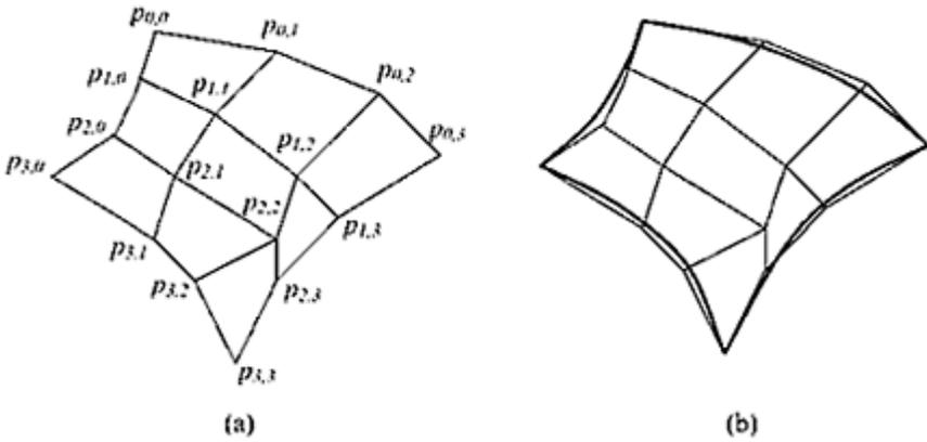
**FIGURE 4.3** (a) A Bézier control net and (b) the resulting cubic Bézier surface patch in tensor product form.
