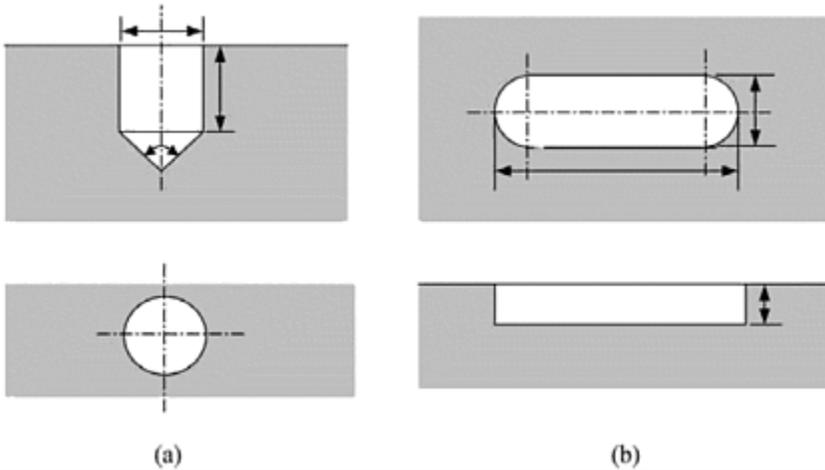
**FIGURE 9.21** Examples of parameterized features. (a) A blind hole with a conical bottom. (b) An elongated slot.
