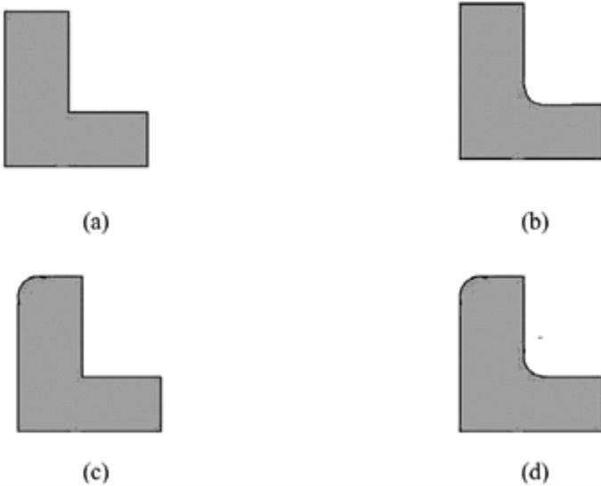
**FIGURE 9.15** (a) A two-dimensional region with sharp corners. (b) Filleting the reentrant (nonconvex) corner. (c) Rounding a convex corner. (d) Applying both rounding and filleting.
