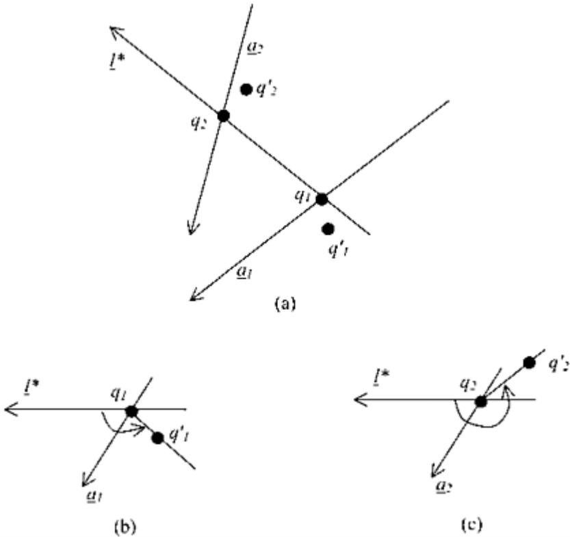
**FIGURE 5.24** Polar coordinate dimensioning employed while dimensioning the relative position of two helices. (a) A general position of the two helices. (b) Polar coordinate dimension for  $q'_1$ . (c) Polar coordinate dimension for  $q'_2$ .
