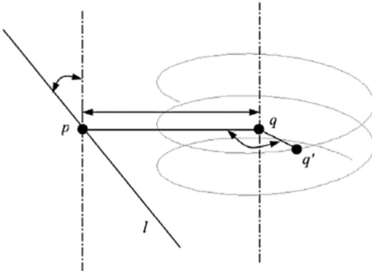
**FIGURE 5.21** Dimensioning the relative position of a line  $l$  and a helix.  $pq$  is the common perpendicular between  $l$  and the axis of the helix. On the helix,  $q'$  is the preimage of  $q$ .
