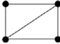
**FIGURE A3.5** A planar five-bar framework that is rigid.
