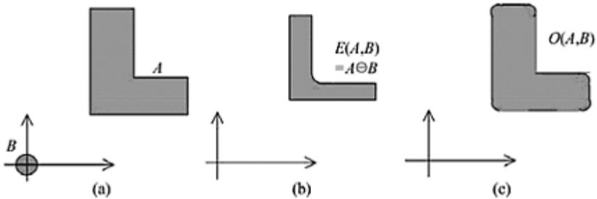
**FIGURE 9.17** Opening  $A$  with  $B$  rounds all sharp (convex) corners. It doesn't affect reentrant (nonconvex) corners.
