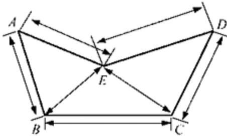
**FIGURE 8.11** Dimensioning a pentagon using seven distance dimensions.
