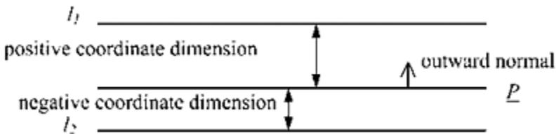
**FIGURE 5.14** Dimensioning the relative position of a nonoriented line and an oriented plane when they are parallel.
