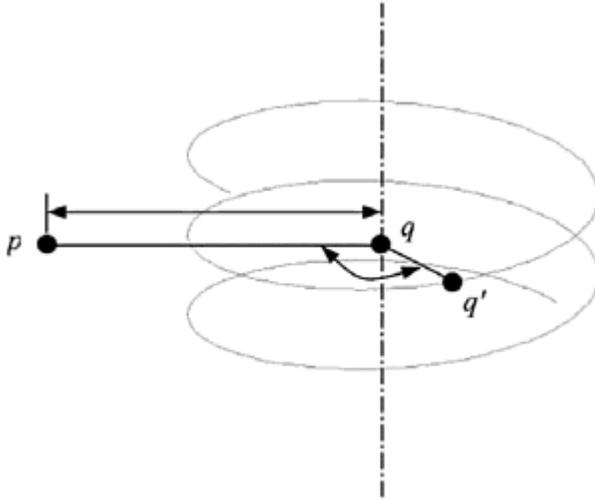
**FIGURE 5.19** Dimensioning the relative position of a point  $p$  and a helix.  $q$  is the projection of  $p$  onto the axis of the helix. On the helix,  $q'$  is the preimage of  $q$ .
