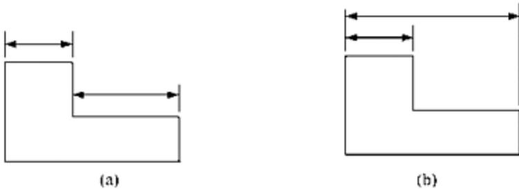
**FIGURE 1.9** A part (partially) dimensioned in two different ways.
