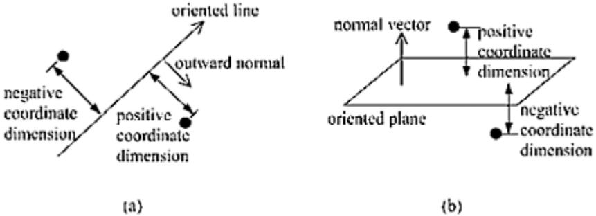
**FIGURE 5.8** Positioning a point relative to (a) an oriented line and (b) an oriented plane. The relative position dimension can have a positive or negative coordinate, depending on which side of the line or plane the point is located.
