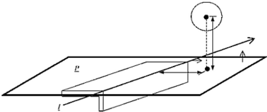
**FIGURE 7.12** Dimensioning the relative position of an infinite bracket (prismatic class) and a sphere (spherical class). The reference tuple for the prismatic class is  $(\underline{P}, \underline{l} \text{ on } \underline{P})$ , where  $\underline{P}$  and  $\underline{l}$  are both oriented. The two dimensions shown are signed and can be considered to be coordinate dimensions.
