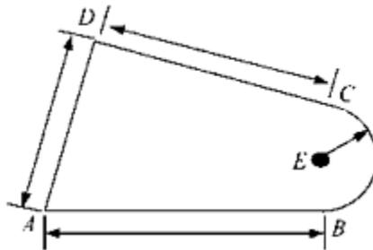
**FIGURE 8.14** A dimensioned planar sketch involving one circular arc.
