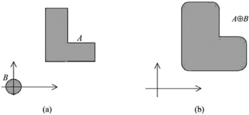
**FIGURE 9.12** Minkowski addition of a two-dimensional region with a circular disk.
