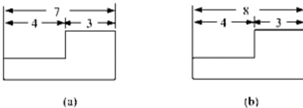
**FIGURE 8.8** (a) Overdimensioning that is consistent. (b) Overdimensioning that is inconsistent.
