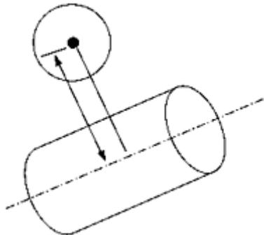
**FIGURE 7.2** Dimensioning the relative position of a member of the spherical class and a member of the cylindrical class.
