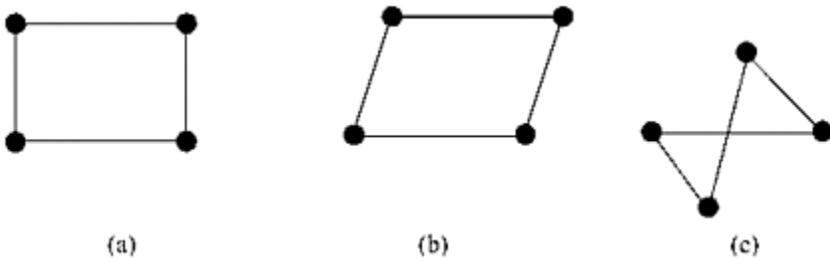
**FIGURE A3.4** A four-bar linkage in the plane in three different configurations.
