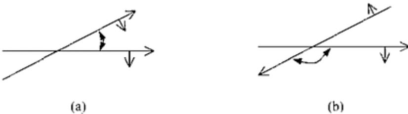
**FIGURE 5.12** Dimensioning the relative position of two intersecting, oriented lines. See also Figure 5.2. Depending on which line is chosen as the origin, the angle dimension indicated can be a positive or a negative dimension.
