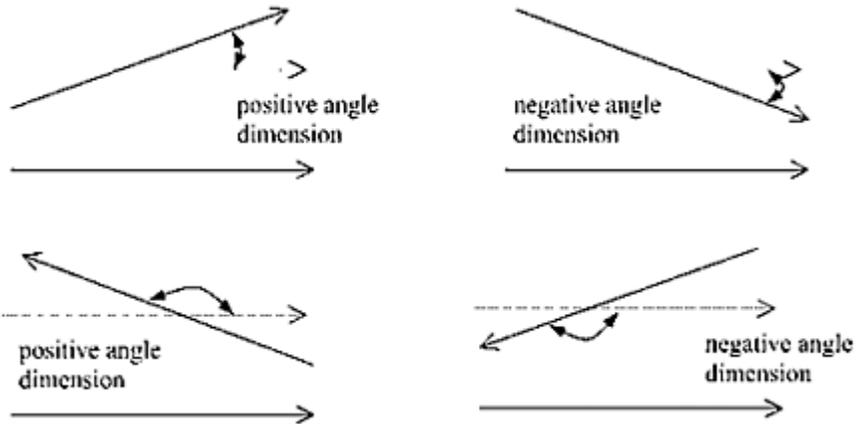
**FIGURE 5.13** Dimensioning the relative position of two oriented, skew lines.
