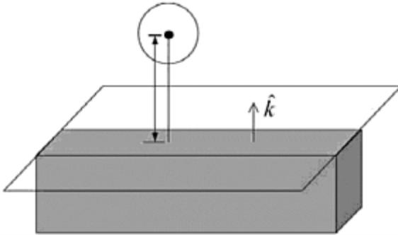
**FIGURE 7.3** Dimensioning the relative position of a member of the spherical class and a member of the planar class. The shaded figure is part of a planar half-space. The bounding plane has an outer normal denoted
