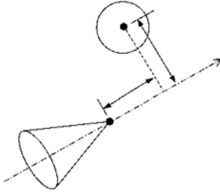
**FIGURE 7.8** Dimensioning the relative position of a sphere and a cone. The dimension from the apex of the cone to the projection of the center of the sphere on to the axis of the cone is a signed value.
