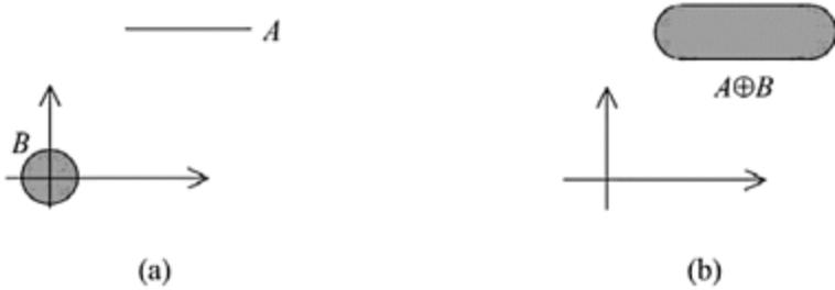
**FIGURE 9.10** Minkowski addition of a line segment and a circular disk.
