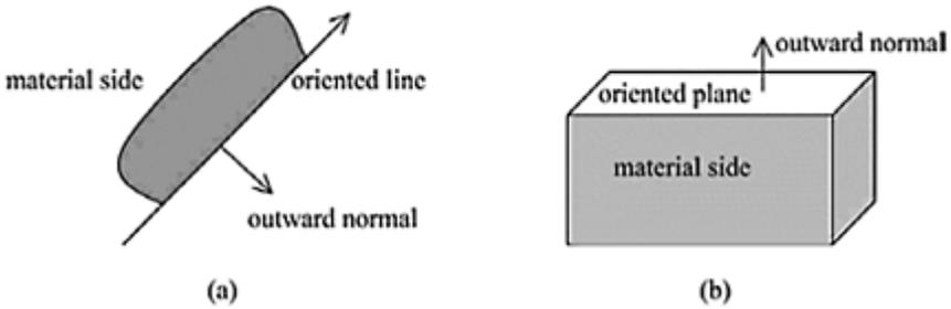
**FIGURE 5.7** Encoding the material side using oriented lines and oriented planes. (a) An oriented line in a plane. The material side is assumed to be on the left of the oriented line. An outward normal is perpendicular to the oriented line and points away from the material side. (b) An oriented plane, whose normal also serves as an outward normal by pointing away from the material side.
