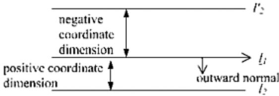
**FIGURE 5.9** Dimensioning the relative position of an oriented line  $l_1$  and a nonoriented line, such as  $l_2$  or  $l'_2$ , when they are parallel.
