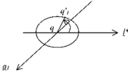
**FIGURE 5.23** Polar angle dimensioning. The polar angle is between the line joining  $q$  and  $q'_1$  and the directed line  $l^*$ . It is measured from the directed line  $l^*$  in the counterclockwise direction determined by the oriented line  $a_1$ .
