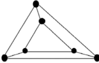
**FIGURE A3.7** A planar nine-bar framework that is rigid.
