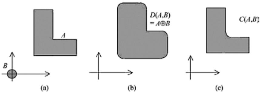
**FIGURE 9.18** Closing  $A$  with  $B$  fillets the reentrant (nonconvex) corner. It doesn't affect convex corners.
