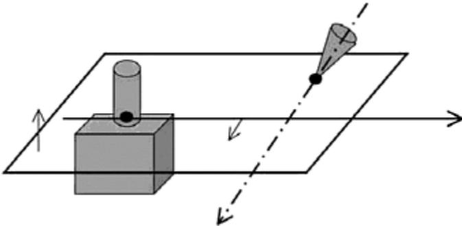
**FIGURE 7.13** Relative positioning a member of the revolute class and a member of the general class.
