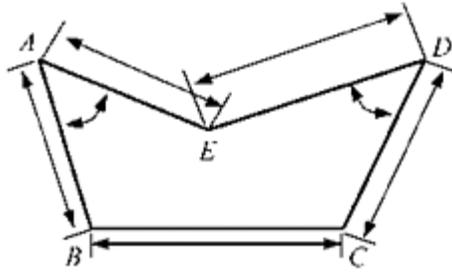
**FIGURE 8.12** Dimensioning a pentagon using five distance dimensions and two angle dimensions.
