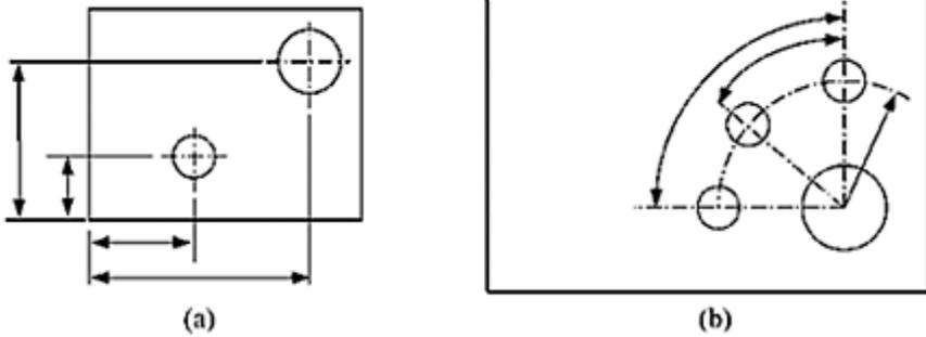
**FIGURE 1.8** (a) Rectangular (Cartesian) coordinate dimensioning. (b) Polar coordinate dimensioning.
