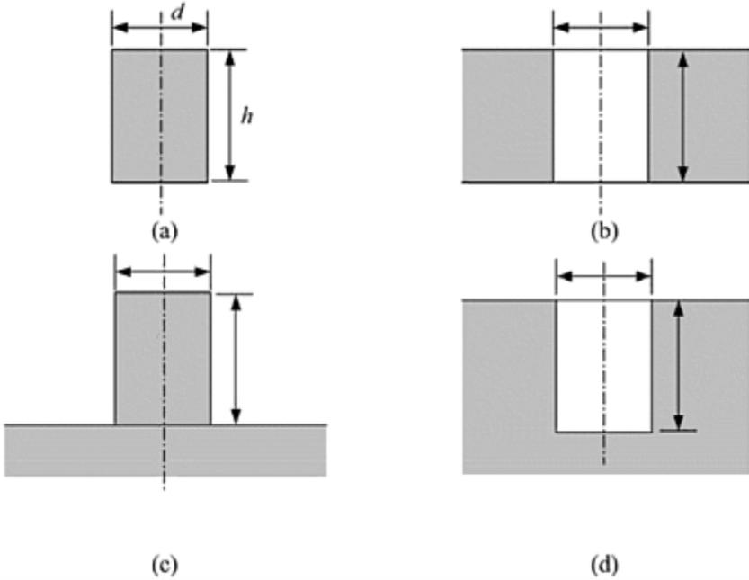
**FIGURE 9.1** Four different solid objects with the same dimensions.
