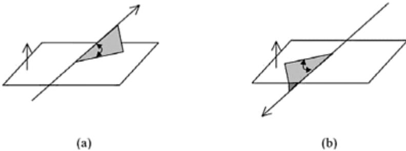
**FIGURE 5.15** Dimensioning the relative position of an oriented line and an oriented plane when they intersect at a point. See Figure 5.5 for comparison. (a) The angle dimension is considered to be a positive dimension because the line orientation has a positive component along the outward normal of the plane. (b) The angle dimension is considered to be a negative dimension because the line orientation has a negative component along the outward normal of the plane.
