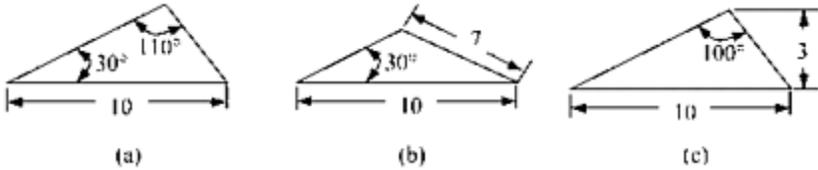
**FIGURE 2.4** Three examples of dimensioned triangles. Are they valid?
