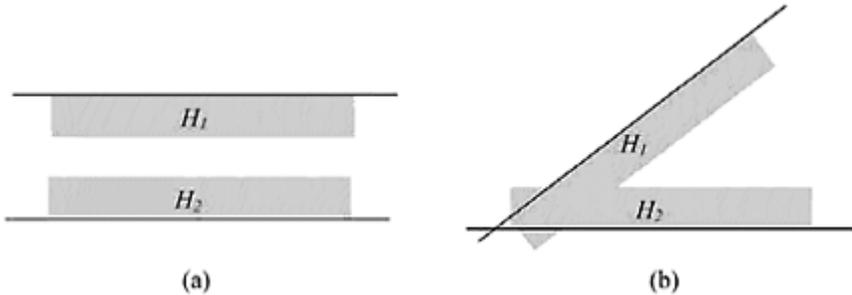
**FIGURE 9.20** Changing the relative positioning of two half-spaces from (a) to (b) in a construction history embodied in the CSG tree of Figure 9.6 (a).
