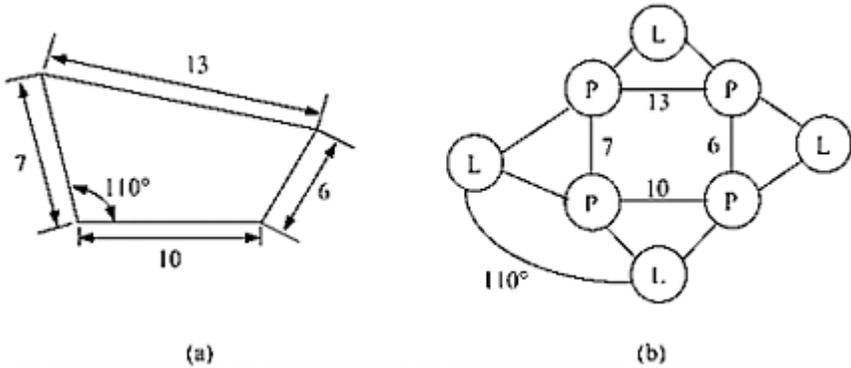
**FIGURE A3.12** (a) A dimensioned quadrilateral, and (b) its dimensional constraint graph.
