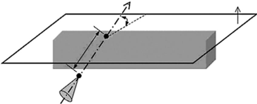
**FIGURE 7.9** Dimensioning the relative position of a conical half-space and a planar half-space. It consists of two dimensions: One is the angle between the oriented axis and the oriented plane, and the other is the distance between the apex of the cone and the point of intersection of the axis with the plane. Both dimensions carry signs, and they happen to be positive in this example.
