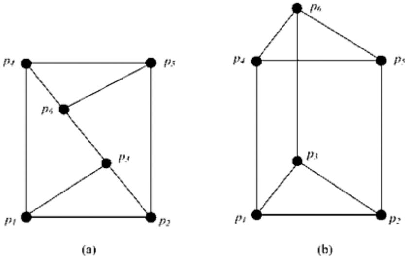
FIGURE A3.10 Two planar nine-bar frameworks.
