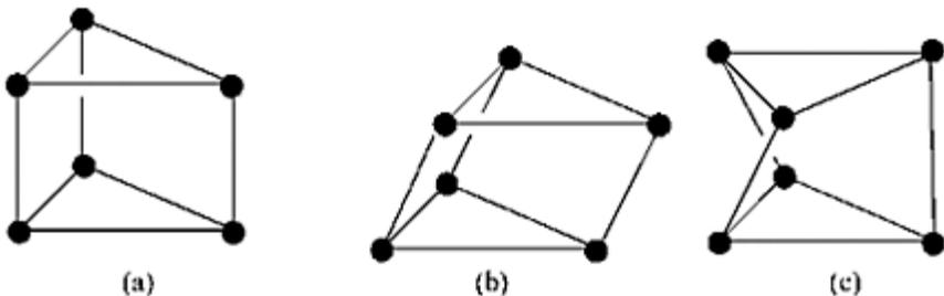
**FIGURE A3.6** A nine-bar linkage in space in three different configurations.
