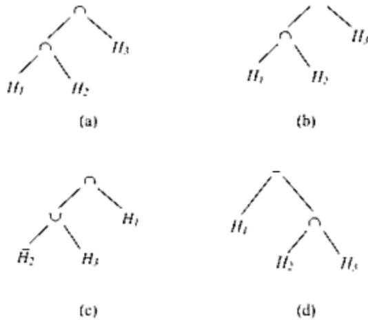
**FIGURE 9.6** CSG tree hierarchy for the construction of each of the solids in Figure 9.1. The half-spaces  $H_1$ ,  $H_2$ , and  $H_3$  are shown in Figure 9.5.
