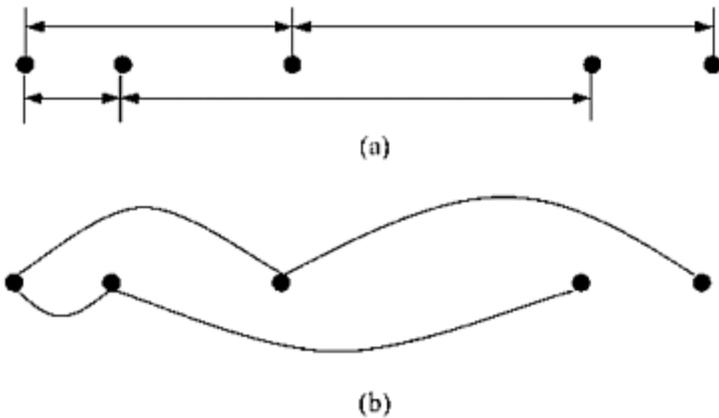
**FIGURE 8.7** (a) Simultaneous dimensioning of relative positions of collinear points. (b) The corresponding dimensional constraint graph.
