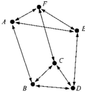
**FIGURE 8.13** Dimensioning a hexagon  $ABCDEF$  using nine distance dimensions.
