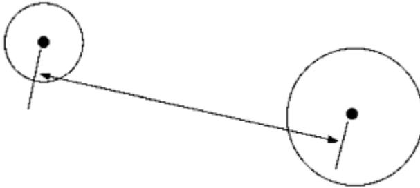
**FIGURE 7.1** Dimensioning the relative position of two members of the spherical class.
