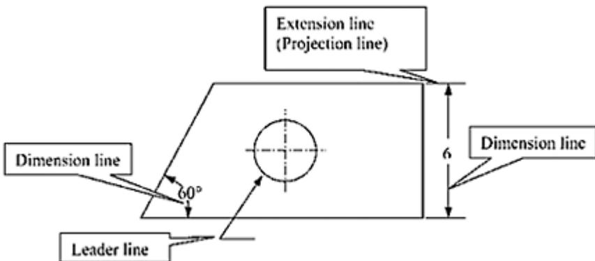
**FIGURE 1.7** Illustration of dimension, extension, and leader lines.
