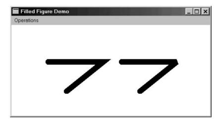
Figure 21-21 Effect of the SetMiterLimit() Function
