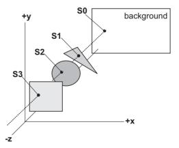
Figure 6-15 Z-Buffer Algorithm Processing
