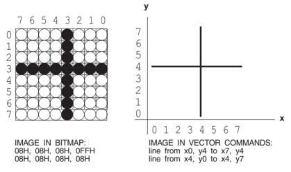
Figure 2-1 Raster and Vector Representation of a Graphics Object
