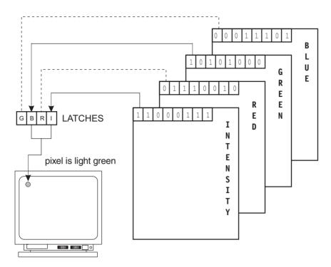
Figure 7-4 Video Memory Mapping in VGA Mode 18
