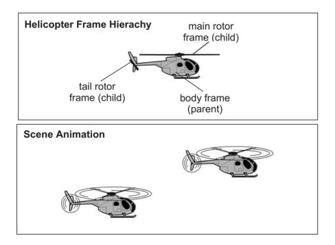
Frame hierarchies in Direct3D are not rigid. Functions are available that enable you to change the reference frame, regardless of the parent-child relationships originally established. This flexibility adds considerable power to retained mode.
