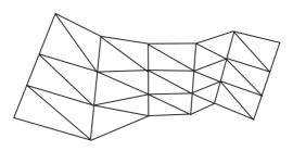
Figure 2-15 Edge Representation of Polygons
