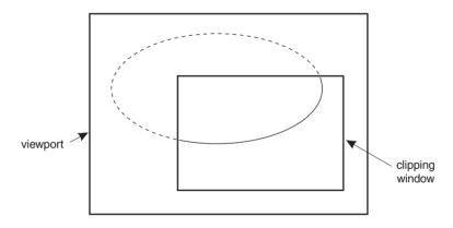
Figure 10-9 Clipping Transformation of an Ellipse
