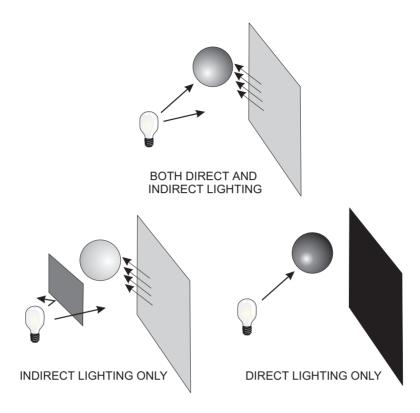
Figure 6-2 Direct and Indirect Lighting
