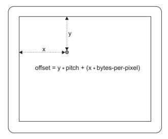
Figure 28-3 Pixel Offset Calculation
