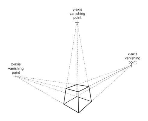
Figure 5-12 Three-Point Perspective of a Cube
