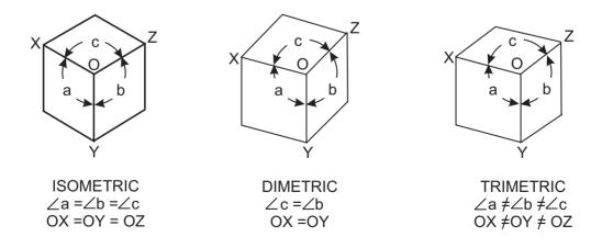
Figure 5-6 Isometric, Dimetric, and Trimetric Projections
