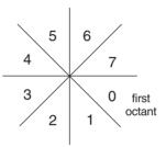
Figure 12-10 Octant Numbering in the Cartesian Plane
