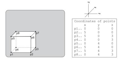
Figure 2-6 3D Representation of a Rectangular Solid
