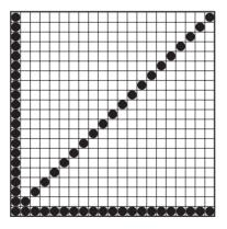
Figure 10-1 Pixel Plots for Straight Lines
