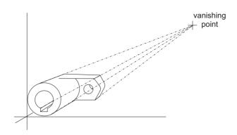
Figure 5-9 One-Point Projection of a Mechanical Component
