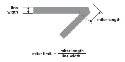
Figure 21-20 Miter Length, Line Width, and Miter Limit
