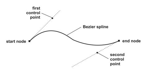
Figure 20-11 Elements of the Cubic Bezier
