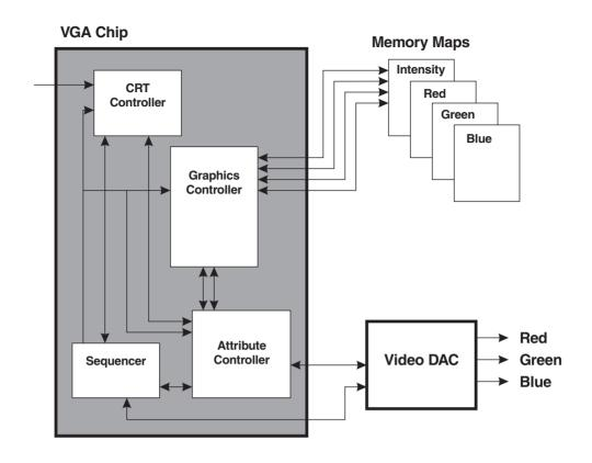
Figure 7-2 VGA System Components
