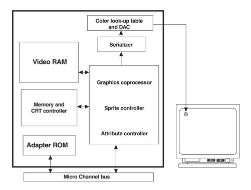
Figure 11-2 XGA Component Diagram
