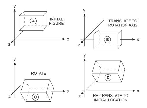
Figure 3-16 Rotation About an Arbitrary Axis
