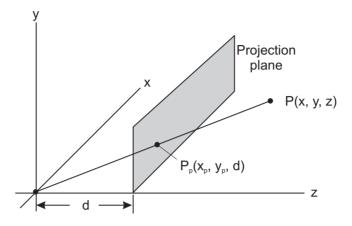
Figure 5-13 Perspective Projection of Point P
