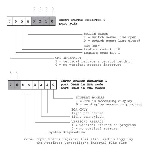
Figure 7-7 VGA Input Status Register
