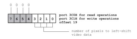
Figure 7-30 Horizontal Pixel Panning Register of the VGA Attribute Controller
