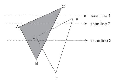
Figure 6-12 Scan-Line Algorithm for Hidden Surface Removal
