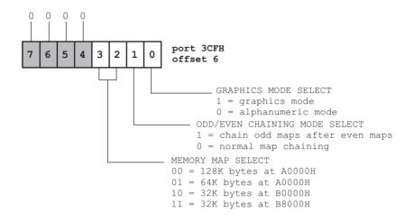
Figure 7-23 Miscellaneous Register of the VGA Graphics Controller
