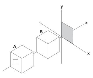
Figure 5-7 Lack of Realism In Isometric Projection
