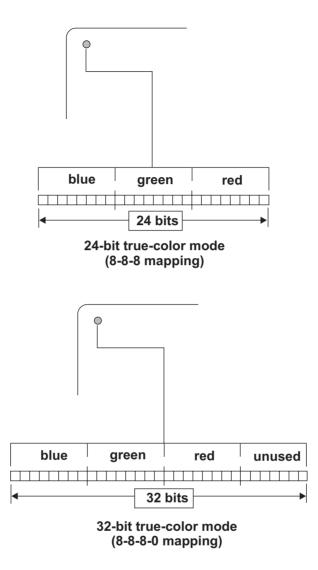
Figure 28-2 Pixel Mapping in True-Color Modes
