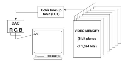
Figure 11-3 Bit Planes in XGA and 8514/A High-Resolution Modes
