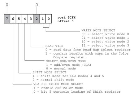
Figure 7-22 Select Graphics Mode Register of the VGA Graphics Controller
