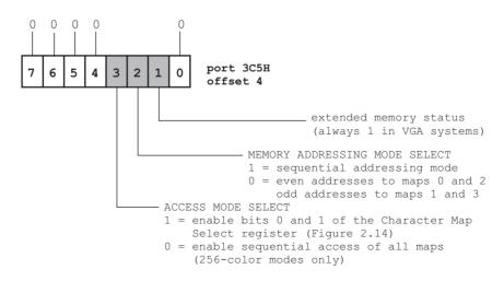
Figure 7-15 Memory Mode Register of the VGA Sequencer
