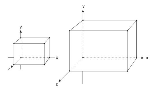
Figure 3-11 Scaling Transformation of a Cube
