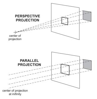
Figure 5-3 Perspective and Parallel Projections
