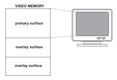
Figure 25-4 Visualization of Primary and Overlay Surfaces
