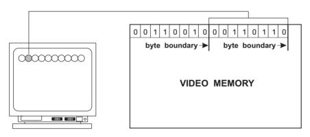
Figure 1-8 Byte-to-Pixel Video Memory Mapping Scheme
