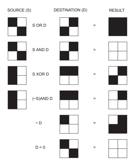
Figure 22-3 Binary and Unary Operations on Bit Blocks
