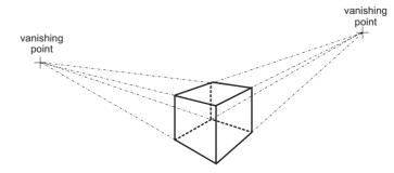
Figure 5-11 Two-Point Perspective of a Cube
