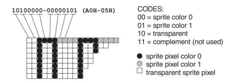
Figure 12-13 Bit-to-Pixel Mapping of Sprite Image
