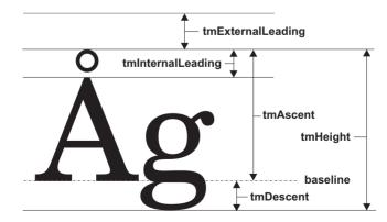
Figure 17-5 Vertical Character Dimensions in the TEXTMETRIC Structure
