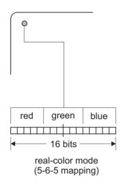
Figure 28-1 Pixel Mapping in Real-Color Modes
