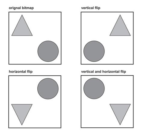
Figure 22-7 Horizontal and Vertical Bitmap Inversion with StretchBlt()
