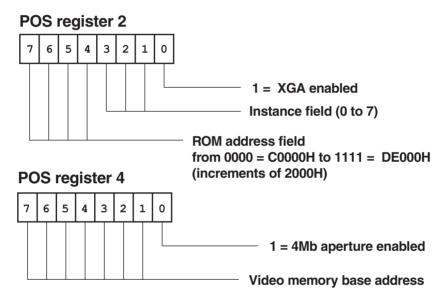
Figure 12-1 XGA Data in POS Registers
