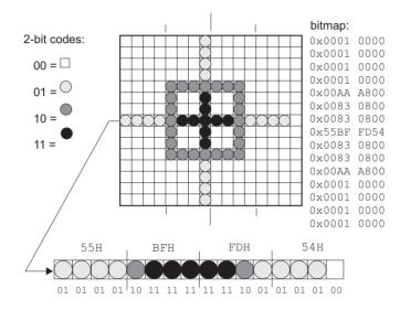
Figure 22-2 Two Bits Per Pixel Image and Bitmap
