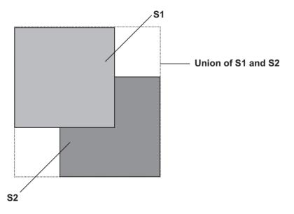
Figure 21-13 Effect of the UnionRect() Function
