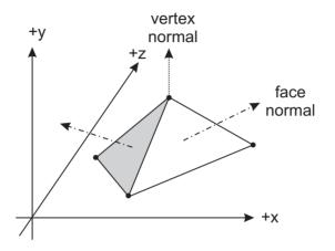
Figure 32-7 Vertex Normals and Face Normals in a Pyramid
