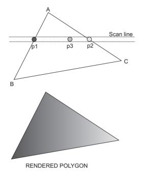
Figure 6-9 Intensity Interpolation in Gouraud Shading
