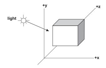
Figure 5-20 Eye Space Transformation of the Cube In Figure 5-17
