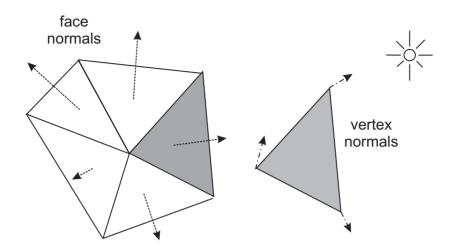
Figure 32-10 Calculating the Vertex Normals
