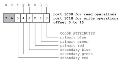
Figure 7-26 Palette Register of the VGA Attribute Controller
