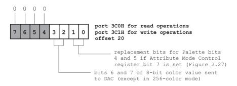
Figure 7-31 Color Select Register of the VGA Attribute Controller
