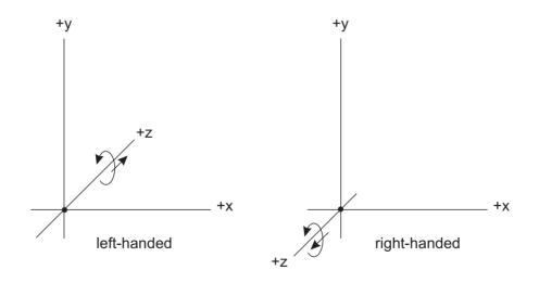
Figure 2-5 Left- and Right-Handed Coordinates
