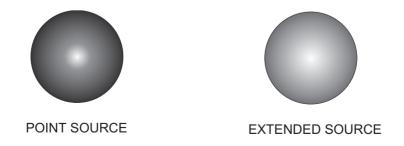
Figure 6-3 Point and Extended Light Sources
