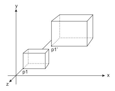
Figure 3-12 Scaling Transformation of an Object Not at the Origin
