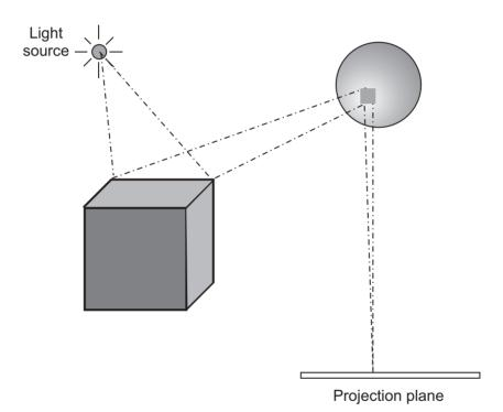
Figure 6-11 Rendering a Reflected Image by Ray Tracing
