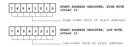
Figure 7-11 Video Start Address Register of the VGA CRT Controller
