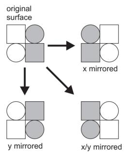
Figure 29-5 Bit-Time Mirroring Transformations
