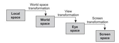
Figure 5-15 Waterfall Model of the Rendering Pipeline
