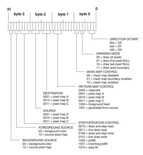
Figure 12-9 Pixel Operations Register Bitmap
