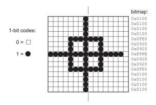
Figure 22-1 One Bit Per Pixel Image and Bitmap
