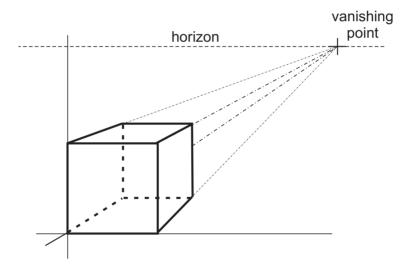
Figure 5-8 One-Point Perspective Projection of a Cube
