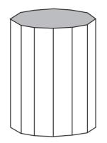
Figure 2-13 Polygonal Approximation of a Cylinder
