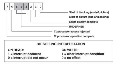
Figure 14-5 XGA Interrupt Status Register Bitmap
