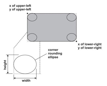
Figure 21-4 Definition Parameters for the RoundRect() Function
