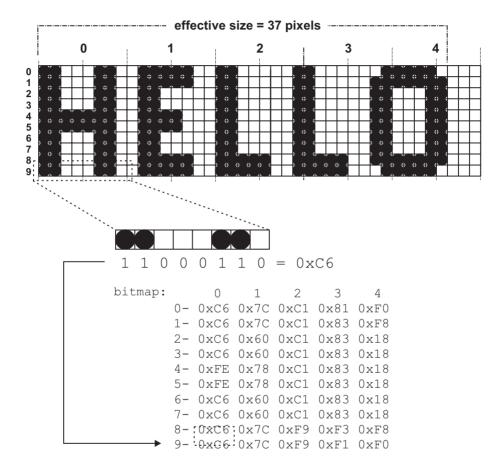
Figure 22-4 Hard-Coded, Monochrome Bitmap
