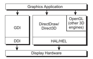
Direct3D provides the API services and device independence required by developers, delivers a common driver model for hardware vendors, enables turnkey 3D solutions to be offered by personal-computer manufacturers, and makes it easy for end-users to add high-end 3D functions to their systems. Because the system requires little memory, it runs well on most of the installed base of computer systems.
