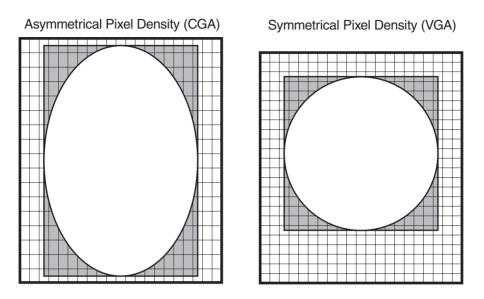
Figure 7-1 Symmetrical and Asymmetrical Pixel Density
