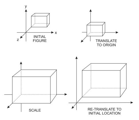
Figure 3-13 Fixed-Point Scaling Transformation
