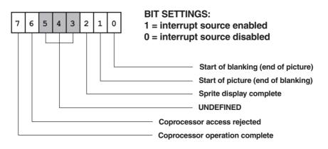
Figure 14-4 XGA Interrupt Enable Register Bitmap
