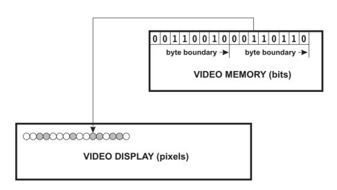
Figure 8-2 Bit-to-Pixel Mapping Example in VGA Mode 18
