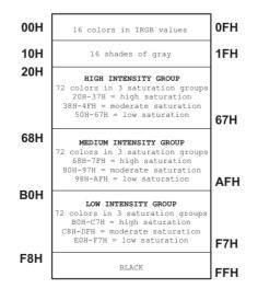
Figure 8-5 Default Color Register Setting in VGA Mode 19
