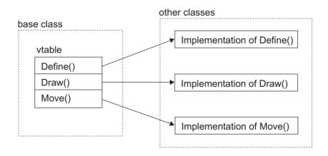
Figure 24-2 The Virtual Function Table (vtable)
