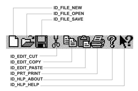
Figure 19-12 "Toolbar.bmp" Button Identification Codes
