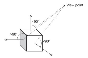
Figure 5-19 Line-of-Sight and Surface Vectors in Culling
