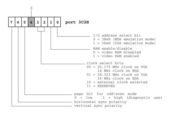
Figure 7-6 VGA/EGA Miscellaneous Output Register
