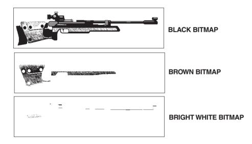
Figure 15-2 Monochrome Overlays to Form a Color Image
