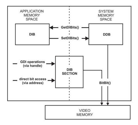
Figure 22-5 Memory Image of Conventional and DIB Section Bitmaps
