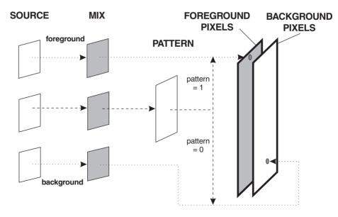
Figure 12-8 Determining the Pixel Attribute
