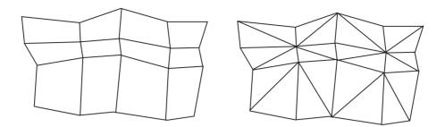
Most graphics systems, including Direct3D, model objects by means of polygon meshes. Mesh information is stored in a database containing the vertices of each polygon and their attributes, such as color, texture, and shading. A state-of-the-art hardware-based renderer is capable of displaying hundreds of thousands to over one million of these polygons in 1 second, and at the same time applying texture, lighting and other effects.
