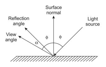
Figure 6-6 Specular Reflection
