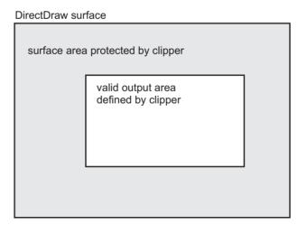
Figure 30-1 Using a Clipper to Establish the Surface's Valid Blit Area.
