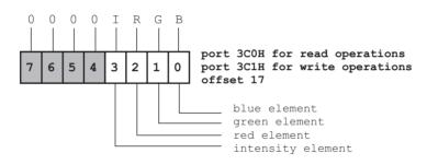
Figure 7-28 Overscan Color Register of the VGA Attribute Controller
