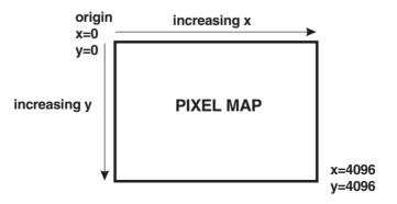
Figure 12-5 Pixel Map Origin and Dimensions
