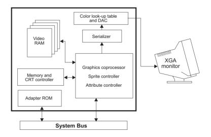
Figure 1-7 XGA Component Diagram
