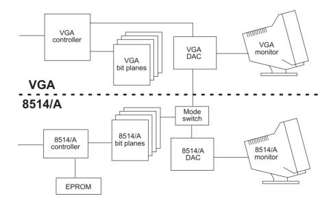
Figure 1-6 Architecture of a VGA/8514A Video System
