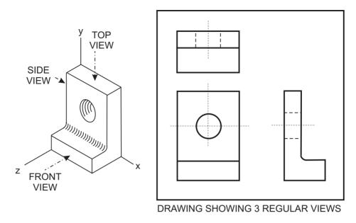
Figure 5-5 Parallel, Orthographic, Multiview Projection
