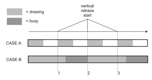
Figure 31-7 Surface Update Time and Frame Rate
