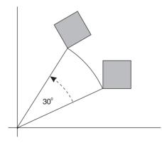
Figure 10-8 Rotation Transformation of a Polygon
