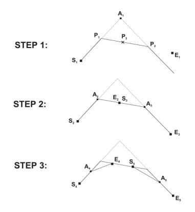
Figure 20-10 Divide-and-Conquer Method of Creating a Bezier Curve
