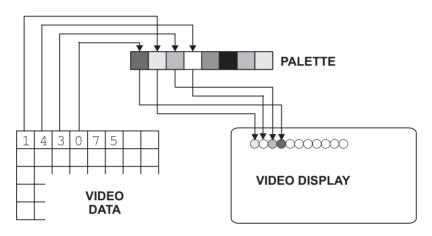
Figure 25-6 Palette-Based Pixel Attribute Mapping
