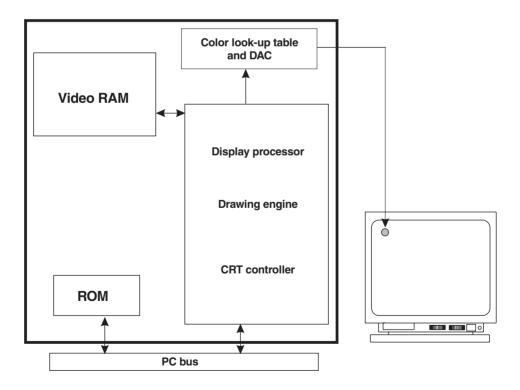
Figure 11-1 8514/A Component Diagram
