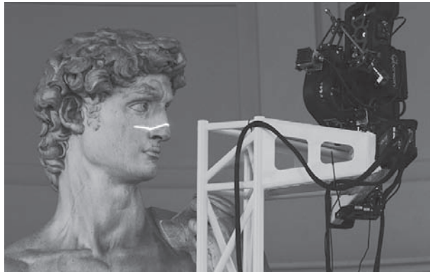
Figure 13.7. Scanning Michelangelo's David. (Courtesy of M. Levoy, Stanford University.)
