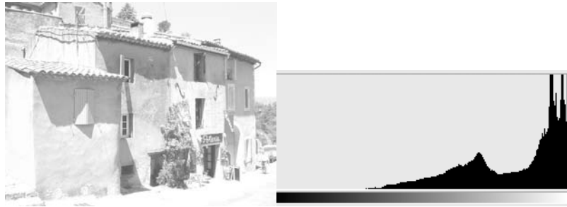
Figure 12.8. An overexposed image (left) and its corresponding histogram (right). The histogram is scaled to a maximum bin size of 31,499 pixels.
