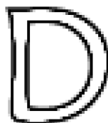
Figure 14.23. Edge detection. A filter is applied to detect a high gradient in the discrete bivariate function (the image). Zooming in on the capital D, we see that the gradient is mapped to a color map with shades of gray.
