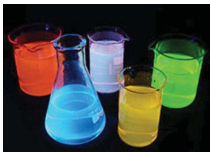
Figure 4.2. Fluorescent solutions under UV-light. Absorbed photons are rapidly re-emitted under longer electromagnetic wavelengths.
