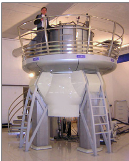
A 900 MHz NMR instrument with a 21.1 T magnet at HWB-NMR.
