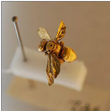
An insect coated in gold for viewing with a scanning electron microscope.
