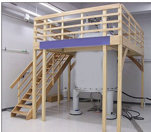
Solid-state 900 MHz (21.1 T) NMR spectrometer at the Canadian National Ultrahigh-field NMR Facility for Solids.
