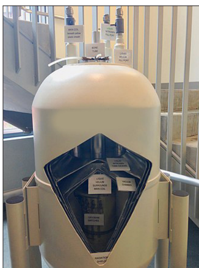
Cutaway of an NMR magnet that shows its structure: radiation shield, vacuum chamber, liquid nitrogen vessel, liquid helium vessel, and cryogenic shims.
