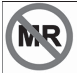
Fig. MR Unsafe Sign.
