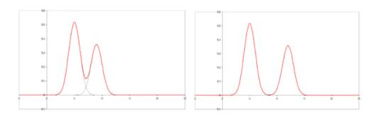
Plotted on the x-axis is the retention time and plotted on the y-axis a signal (for example obtained by a spectrophotometer, mass spectrometer or a variety of other detectors) corresponding to the response created by the analytes exiting the system. In the case of an optimal system the signal is proportional to the concentration of the specific analyte separated.
