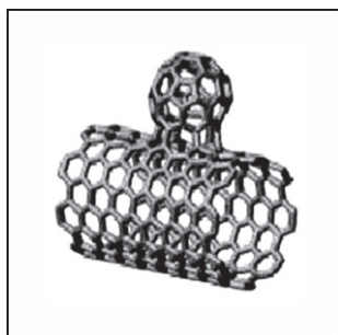
Figure: A Stable Nanobud Structure
