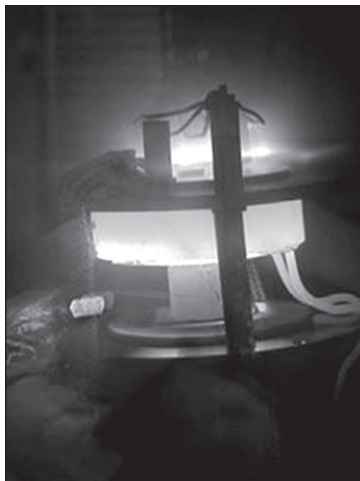
Figure: Nanotubes being grown by Plasma Enhanced Chemical Vapour Deposition
