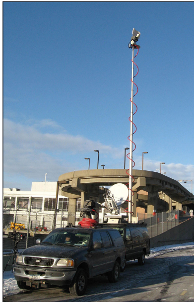
Production truck used for remote broadcasts by television news has a microwave dish on a retractable telescoping mast to transmit live video back to the studio.
