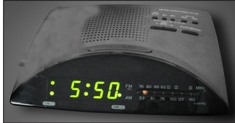
A bedside clock radio that combines a radio receiver with an alarm clock.
