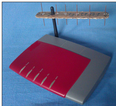
Yagi-Uda antennas, widely used for television reception, are relatively compact at Wi-Fi wavelengths.
