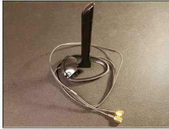
Antenna of wireless network interface controller Gigabyte GC-WB867D-I. Simple stick-like antennas like these have unidirectional reception and relatively low range of 20m or so.
