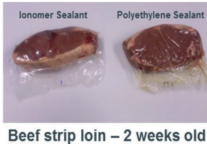
Figure 2. Vacuum packages with polyethylene and ionomers as sealants and the combined effect of secondary seal and protein adhesion.
