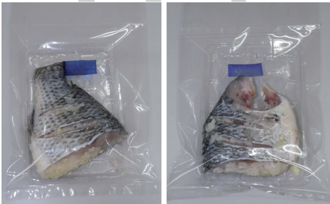
Figure 5. Example of freshness indicator for monitoring the degree of fermentation of plaa-som, a Thai fermented fish. The indicator produced from gelatin film incorporated with anthocyanins extracted from butterfly pea (left) and gelatin film containing rezasurin (right).
