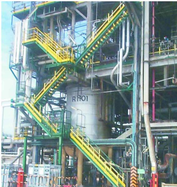
A CSTR reactor, used to make poly(ethene) in bulk.
