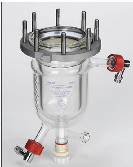
A reaction vessel: Notice there is actually a glass inside another and the other glass contain is used to allow cooling liquids to flow through.
