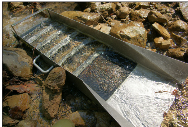
A modern sluice box made of metal; in its base are the riffles used to catch gold settling to the bottom.
