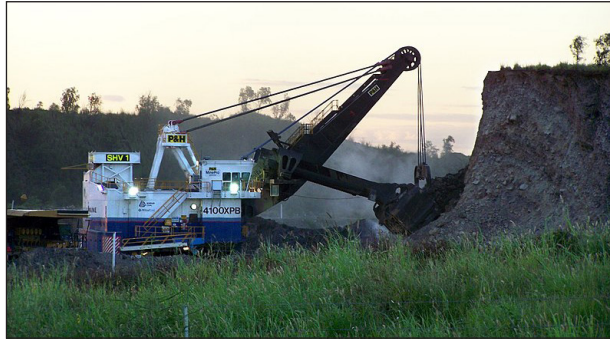
Shovel digging overburden.
