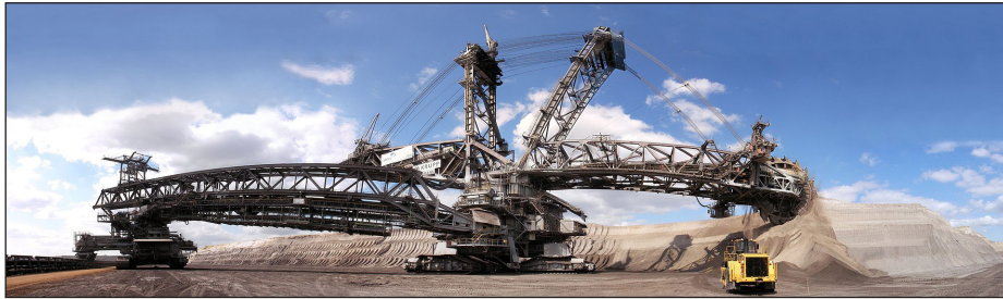
The Bagger 288 is a bucket-wheel excavator used in strip mining. It is also one of the largest land vehicle of all time.
