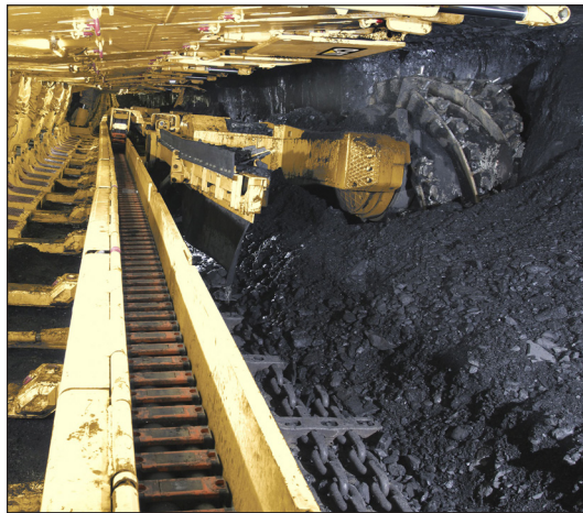
A longwall miner shearing coal at the face of a coal seam.
