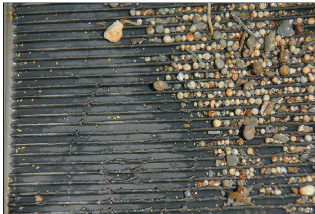
Riffles in a sluice box. The small specks are gold, the larger ones are merely pebbles.
