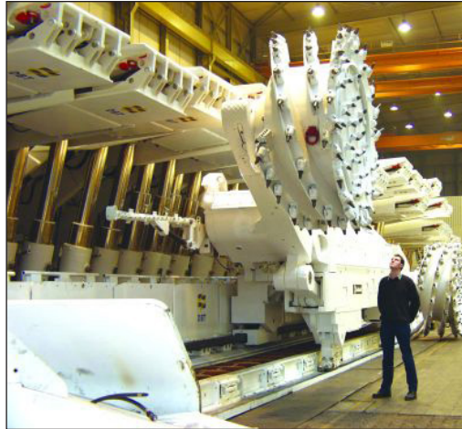
Hydraulic chocks, conveyor and shearer.
