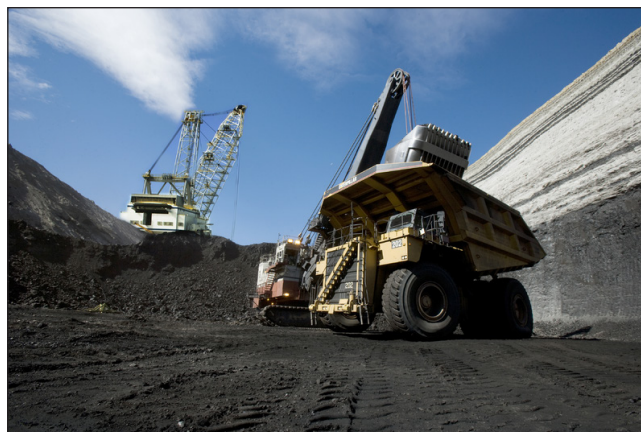
A Bucyrus Erie 2570 dragline and CAT 797 haul truck at the North Antelope Rochelle opencut coal mine.
