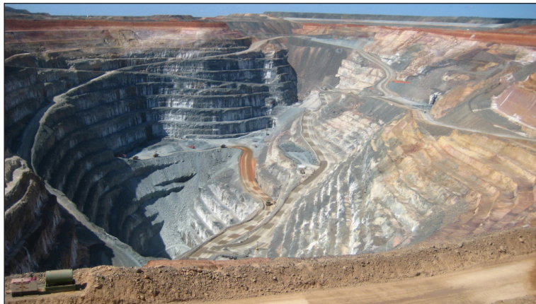
Note the angled and stepped sides of the Sunrise Dam Gold Mine, Australia.
