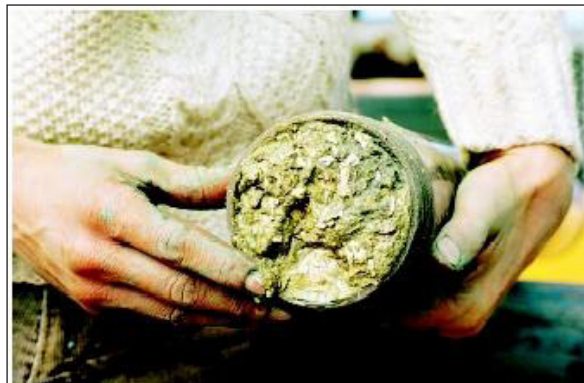
A core sample of sediment from Chesapeake Bay can tell scientists about the oceanographic history of that particular location, including climate change, pollution, and past changes in erosion.
