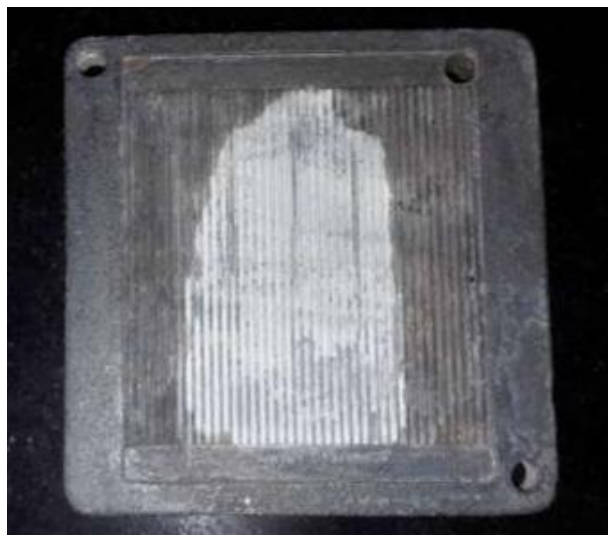
Fig. 9. White channels were not used during methanol dehydration
