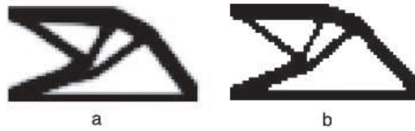
Figure 17. The final topology of a cantilever beam: (a) MMA and (b) BESO.
