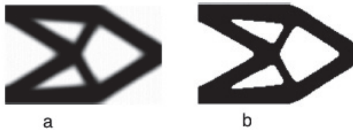
Figure 11. The final topology of a short cantilever beam: (a) \alpha = 0.5 and (b) \alpha = 1.0 .
