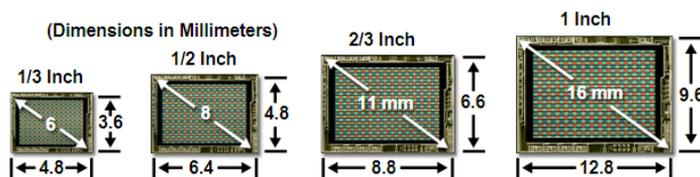
Figure 4. Common CCD image sensor formats.
