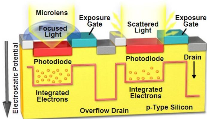
Figure 8. Microlens Array Interline CCD Technology.
