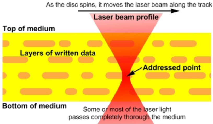
Schematic representation of a cross-section through a 3D optical storage disc (yellow) along a data track (orange marks). Four data layers are seen, with the laser currently addressing the third from the top. The laser passes through the first two layers and only interacts with the third, since here the light is at a high intensity.
