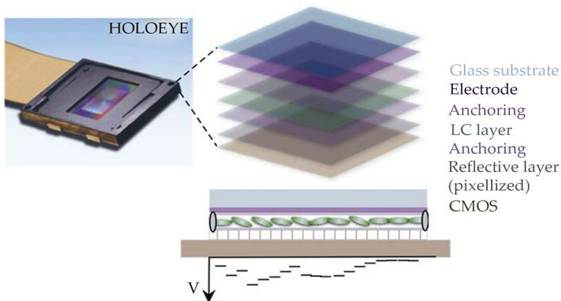
**Figure 3:** Structure and cross-section of an LCoS SLM and photograph of an industrial product from Holoeye.
