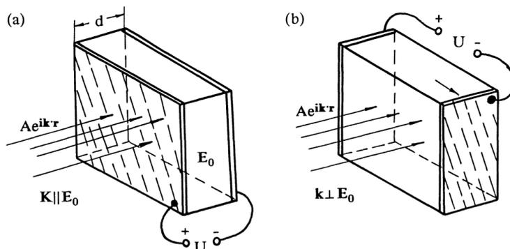
**Figure 3.** Mutual orientations of the applied electric field  $E_0$  and light propagation direction (direction of  $K$ .) for (a) the longitudinal electro-optic effect, and (b) the transverse electro-optic effect.
