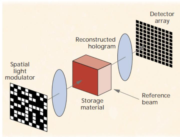
**Figure 2.** For data storage, information is put onto the object beam with a spatial light modulator and removed from a reconstructed object beam with a detector array.
