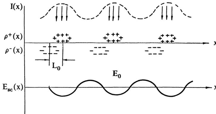
**Figure 2.** Formation of charge and electric-field gratings in a photorefractive crystal through drift.
