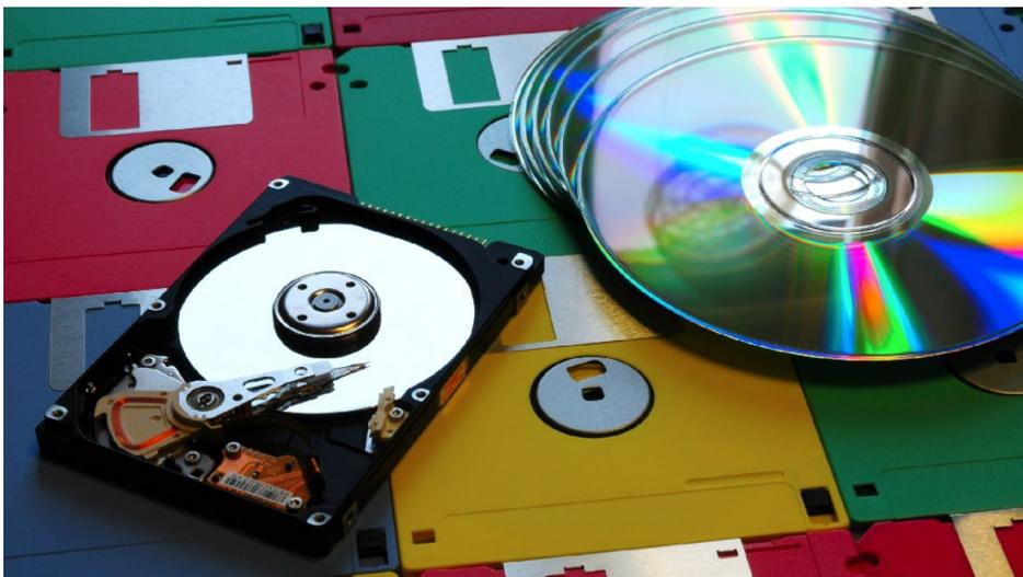
Optical memory was developed by Philips and Sony and released in 1982 in the fourth generation of computers. These memories use light beams for its operations and require optical drives for its operations. These memories are used for storing audio/video, backup as well as caring for data. Read/write speed is slower compared to hard disk and flash memories. Examples
