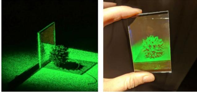
Unless the physical structure is chemically manipulated the reflection hologram will appear the color that it is recorded. To create a true color reflection hologram a multiple laser colors are combined – usually a red, green and blue.
