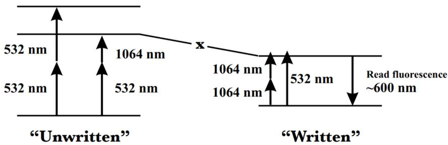
Figure 5. Energy band diagrams for the unwritten and written forms of the fluorescent photochromic material spiropbenzopyran.
