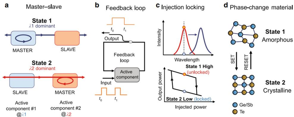
**Figure 2.** Optical memory bistability based on different approaches. **a** master-slave scheme, **b** feedback loop scheme, **c** injection-locking technique and **d** phase-change material (PCM) properties in the case of GST compounds
