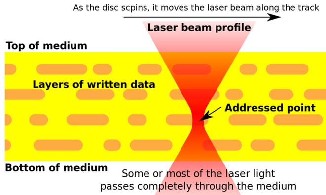
**Figure 1:** A schematic diagram showing a cross-section of an optical 3D storage.
