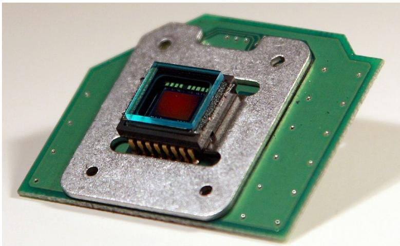
The interline architecture extends this concept one step further and masks every other column of the image sensor for storage. In this device,
