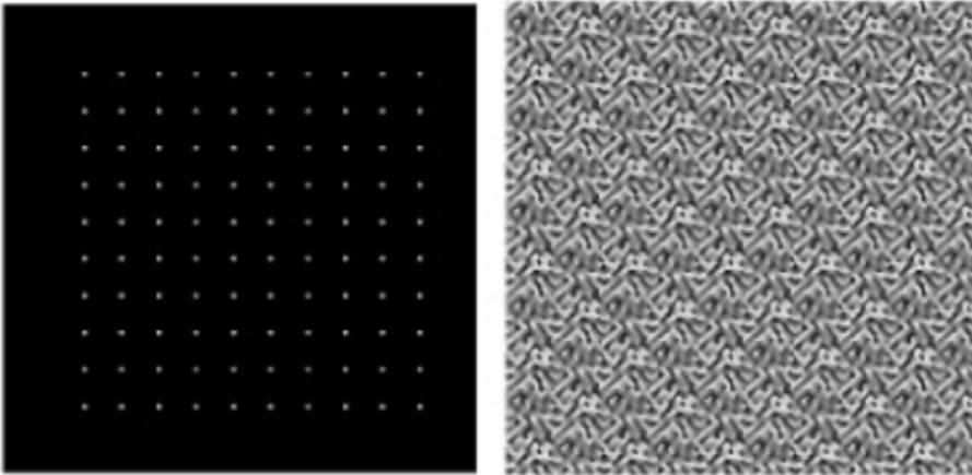
**Figure 4:** Holograms for a  $10 \times 10$  square array of traps generated using the GS algorithm. (a) Input image (b) Generated phase hologram
