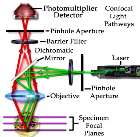
Confocal Microscope Scanning Systems - Confocal imaging relies upon the sequential collection of light from spatially filtered individual
