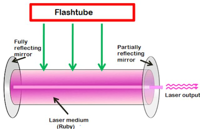
In solid-state lasers, light energy is used as pumping source. Light sources such as flashtube, flash lamps, arc lamps, or laser diodes are used to achieve pumping.
