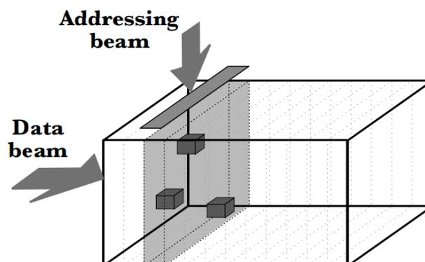
**Figure 4.** Orthogonal beams used to write and read data in parallel in 3-dimensions using 2-photon fluorescence.
