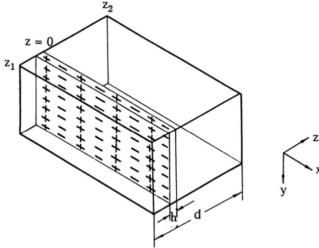
**Figure 5.** Thin charge grating in a crystal of thickness  $d$  (grating thickness:  $h \ll d$ ).
