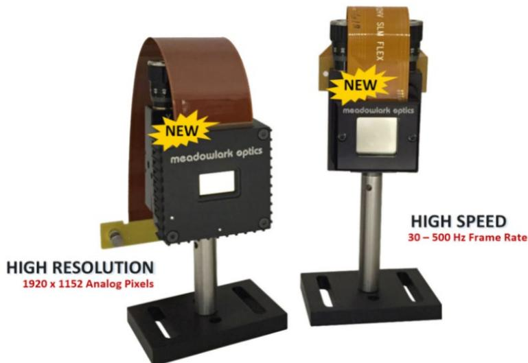
The use of LC materials in SLMs is based on their optical and electrical anisotropy. A certain gray level represents a defined average voltage across the LC cell. This voltage leads to a variable tilt of the LC molecules due to their electrical anisotropy. As LC molecules also show optical
