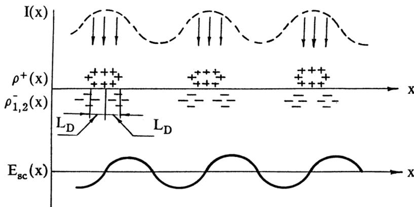
**Figure 1.** Formation of charge and electric-field gratings through diffusion on illumination by the recording light.
