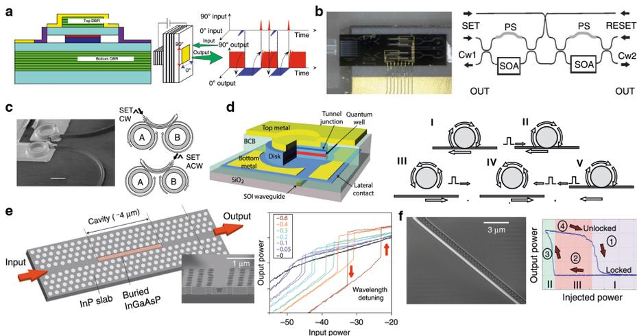
**Figure 3.** Optical memory devices and their respective principle of operation. **a** VCSEL-based optical memory, **b** an SOA-MZI coupled optical memory, **c** an InP micro-ring laser memory, **d** an InP microdisk memory, **e** an InGaAsP photonic crystal nanocavity memory and **f** an InP-on-SOI hybrid photonic crystal nanocavity laser memory.
