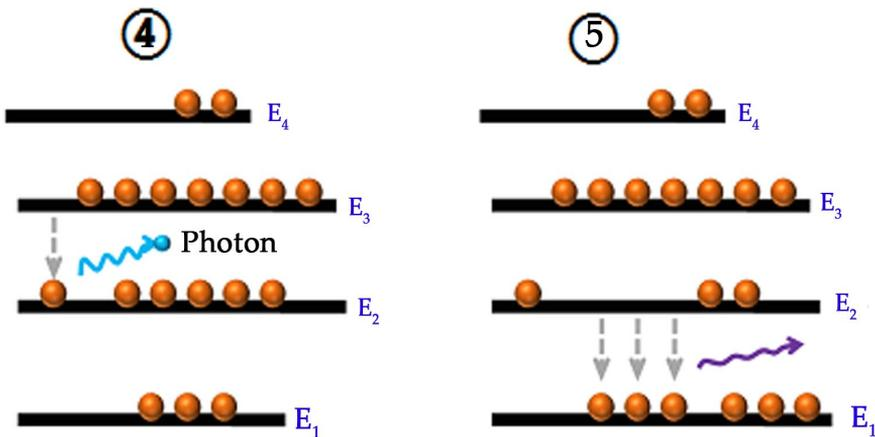
The lifetime of energy state  $E_2$  is very small just like the energy state  $E_4$ . Therefore, after a short period, the electrons in the energy state  $E_2$  will fall back to the ground state  $E_1$  by releasing radiationless energy.
