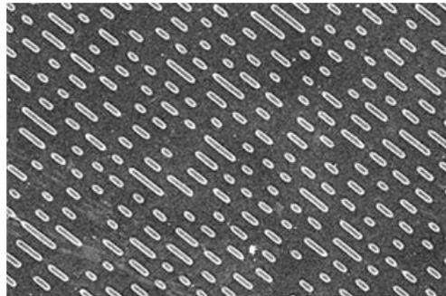
The information on the Compact Disc is recorded in digital form as a spiral track consisting of a succession of pits.
