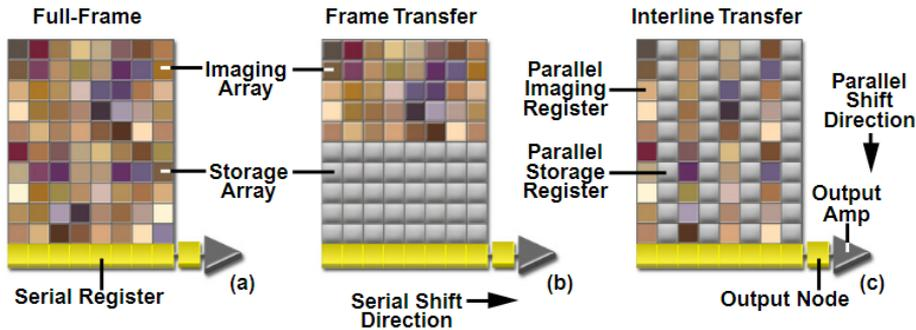
Figure 7. Common charge-coupled device (CCD) architectures.
