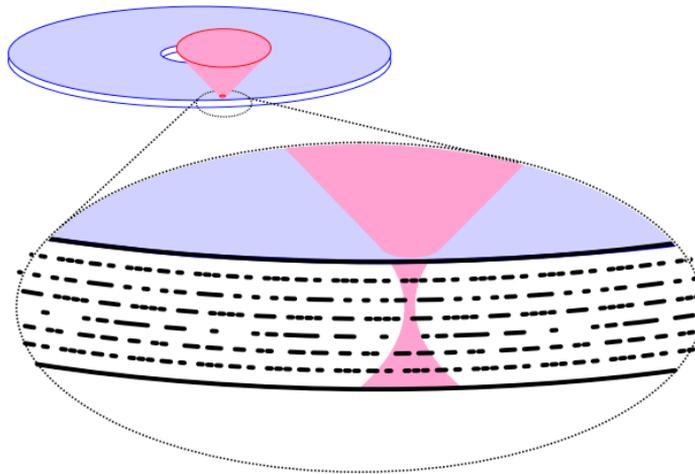
**Figure 3.** Bits are localized within a initially homogeneous block of media by careful focusing and either confocal imaging, nonlinear material response, or both.
