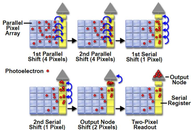
Figure 9. 2 x 2 Pixel Binning Electron Transfer Sequence.
