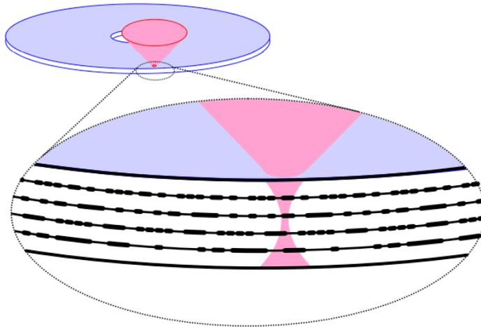
**Figure 2.** A pre-fabricated disk with multiple layers is accessed from one surface for bit-localized volumetric optical storage.
