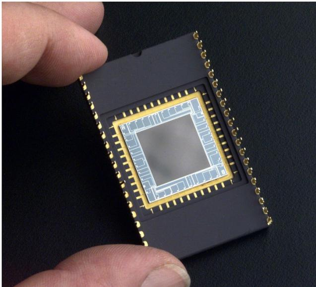
In a CCD image sensor, pixels are represented by p-doped metal–oxide–semiconductor (MOS) capacitors. These MOS capacitors, the basic building
