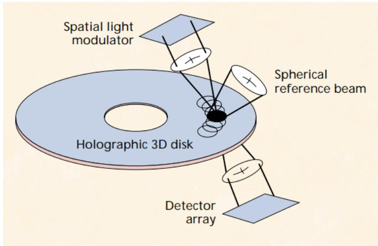
**Figure 5.** A shift-multiplexed disk resembles a compact disk, with an SLM and detector array for parallel input/output, and a simple reference beam. Track position and disk rotation enable access to densely overlapped holograms.
