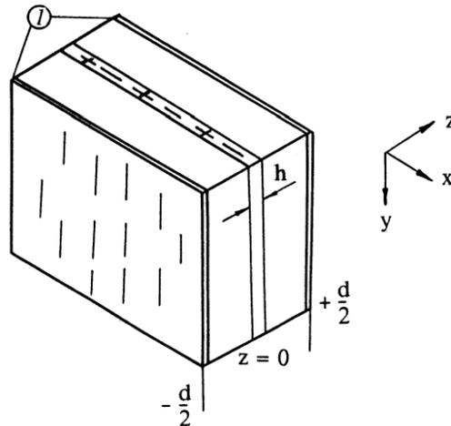
**Figure 6.** Thin charge grating in the center of a crystal. The front and back faces of the crystal are coated with electrodes.
