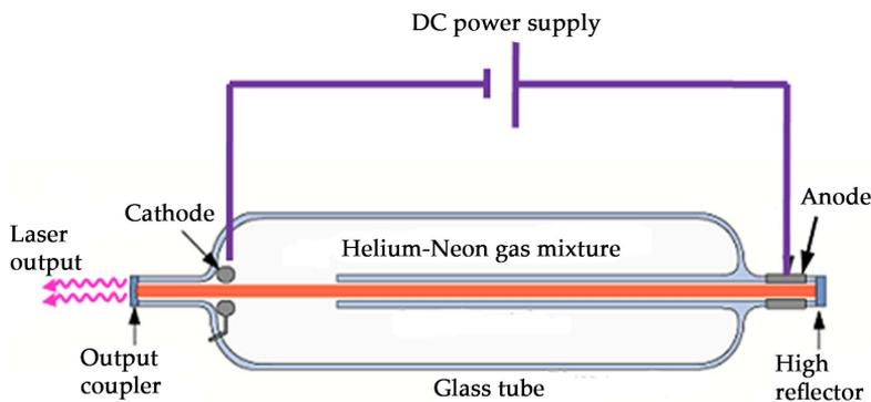
Gas lasers are used in applications that require laser light with very high beam quality and long coherence lengths.
