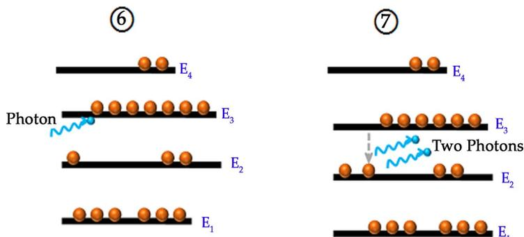
When these two photons again interacted with the metastable state electrons, four photons are released. Likewise, millions of photons are emitted. Thus, optical gain is achieved.
