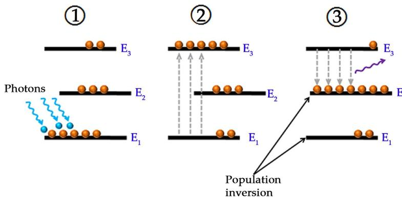
When light energy is supplied to the laser medium (ruby), the electrons in the lower energy state or ground state ( $E_1$ ) gain enough energy and jump into the pump state ( $E_3$ ).
