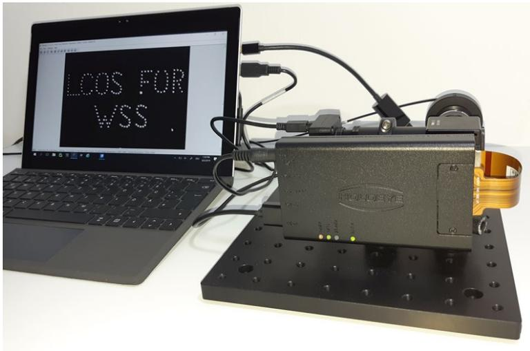
A spatial light modulator is an electronically programmable device that can modulate light output based on a specific fixed spatial pattern (pixel), essentially projecting light that is controlled in either amplitude only, phase only or both (phase-amplitude). This device makes use of liquid crystals to modulate the light, which is why overhead projectors are called LCD projectors.
