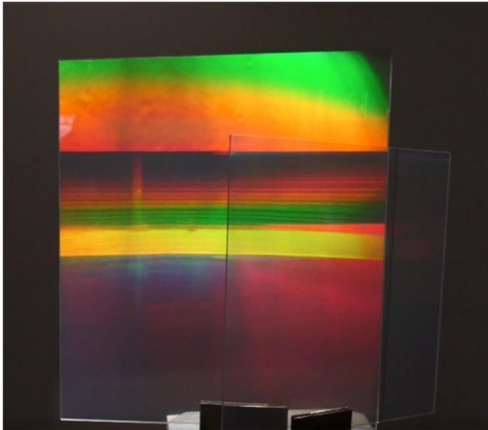
A rainbow hologram, recorded from a horizontal master strip and replayed with a light from above, will have horizontal parallax – enabling the spatial qualities when looking with two eyes or moving side-to-side. But moving up-and-down produces no change in spatial perspective and viewer only sees a change of color. By recording a number of masters on
