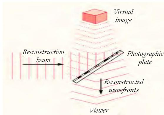
The viewer can move his or her viewpoint and see the image rotate exactly as the original object would. The central miracle of holography is that when the recorded grating is later illuminated by a substitute reference beam, the original object beam is reconstructed, producing a 3D image.
