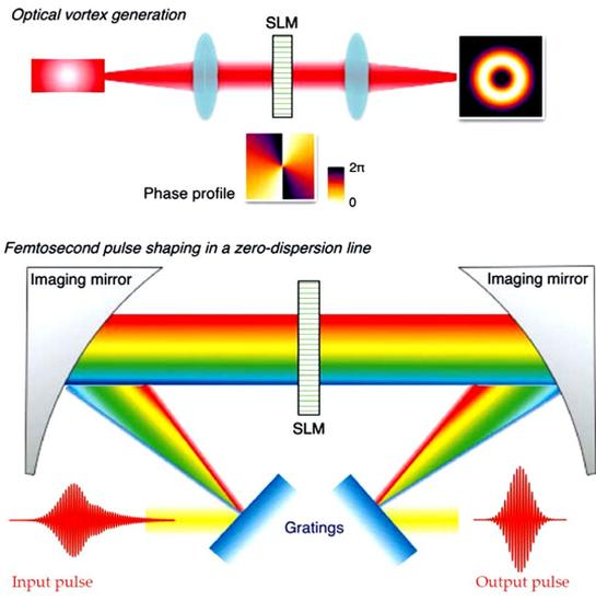
**Figure 2:** Illustration of some applications of SLMs. Top: a spiral phase pattern leads to optical vortex beams. Bottom: a SLM inserted in a zerodispersion line enables the temporal shaping of a femtosecond pulse.
