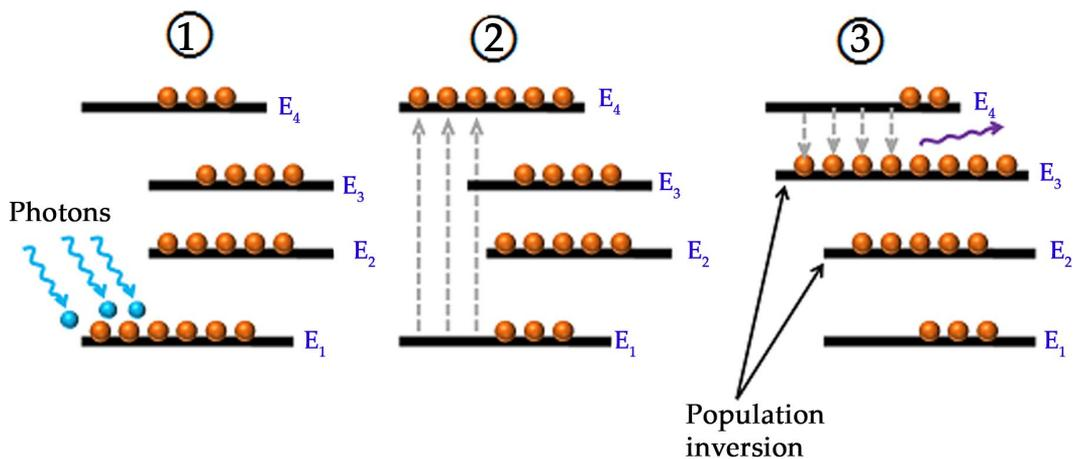
The lifetime of pump state or higher energy state  $E_4$  is very small (230 microseconds ( $\hat{A}\mu s$ )) so the electrons in the energy state  $E_4$  do not stay for long period. After a short period, the electrons will fall into the
