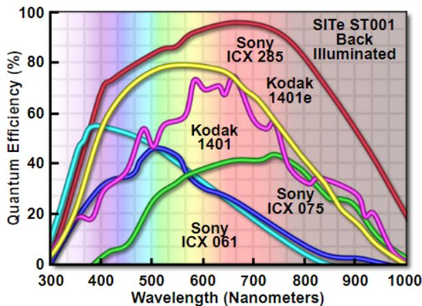
Figure 10. Scientific CCD Spectral Sensitivities.
