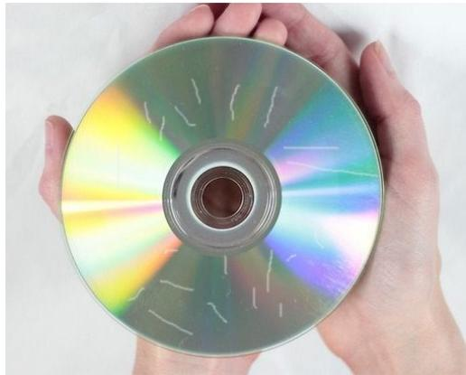
When the laser falls on a scratched spot, it scatters, even if there is no bump at this point. As a result, the photocell transmits incorrect information to the circuit, making it difficult for the CD player to read the data correctly.
