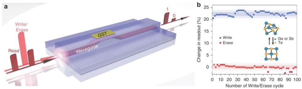
**Figure 4.** Optical phase-change memory device and its respective principle of operation. a Information is stored in the phase state of the GST section on top of the nanophotonic waveguide. b Demonstration of binary memory operation between the crystalline (lower, level 0) and amorphous (upper, level 1) states of a 5  $\mu\text{m}$  GST device for multiple repetitions of the same switching cycle.
