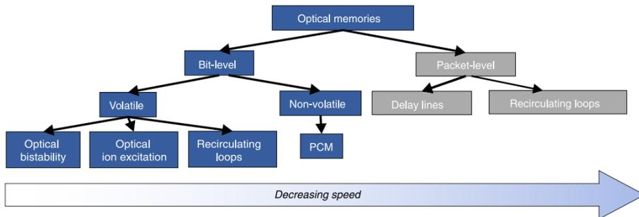
**Figure 1.** Classification of optical memory technologies
