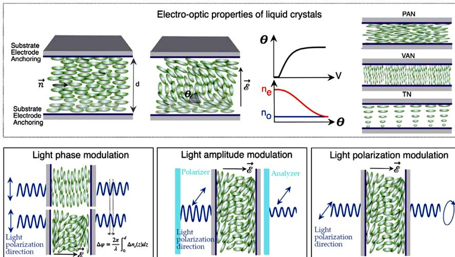
**Figure 1:** Electro-optical properties of nematic liquid crystal layers enable to locally change the phase of the propagating readout light.
