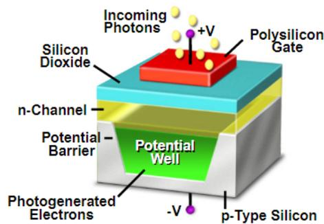
Figure 2. Metal oxide semiconductor (MOS) capacitor.
