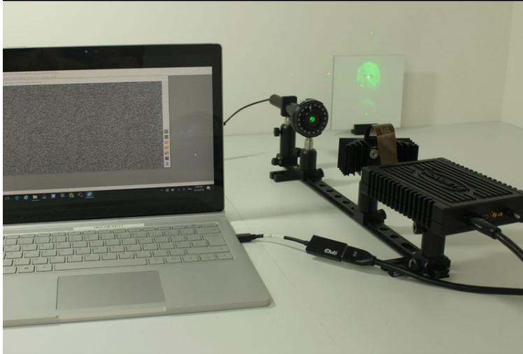
A spatial light modulator (SLM) is a special device that can manipulate light by modulating the amplitude, phase or polarization of the light waves in the two dimensions of space and time. This means that light is manipulated in order to obtain a desired output, and SLM is commonly used in overhead projectors such as those used in schools and office conference rooms.
