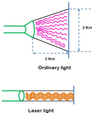
If an ordinary light travels a distance of 2 km, it spreads to about 2 km in diameter. On the other hand, if a laser light travels a distance of 2 km, it spreads to a diameter less than 2 cm.
