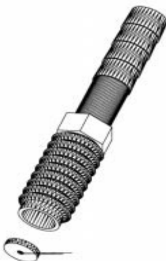
Figure: Drawing of PVC tubing connector with restriction orifice
