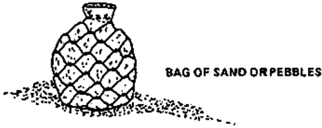
Figure: Types of anchor used for floating cages
