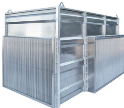
Figure: Oxygen platform for dissolving pure oxygen at low pressure while pumping water around in the farm. The system typically increases the level dissolved oxygen to just above 100% when entering the fish tanks depending on flow rates and farm design
