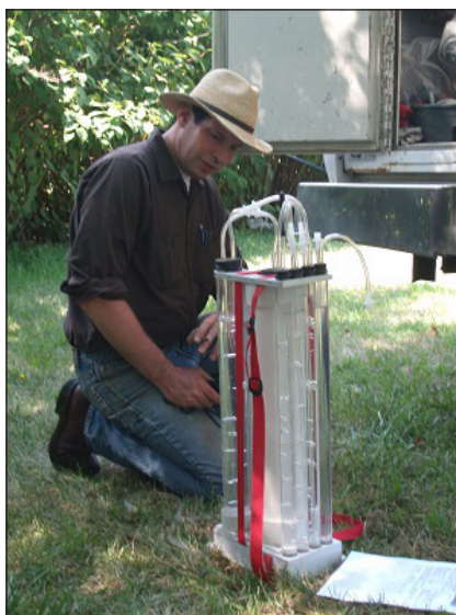
Measuring saturated hydraulic conductivity This is a device (Amoozemeter) that measures how fast water flows in the ground.
