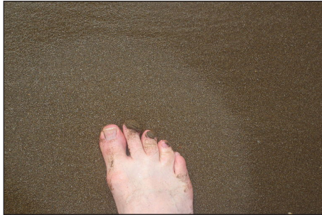
Foot pressure on sand causes it to dilate, drawing water from the surface into the pores.
