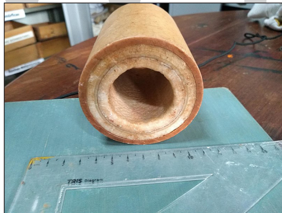
Saline incrustation in a PVC irrigation pipe from Brazil.
