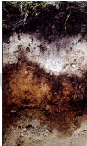
Podzol soil profile from Ireland, showing a bleached layer from which humus and metal oxides have been leached and subsequently deposited in the typically reddish horizon.
