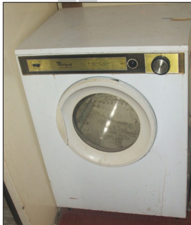
Electric clothes dryer, which is open loop controlled by running the dryer for a set time, regardless of clothes dryness.
