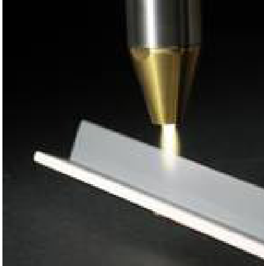
Plasma beam cleaning a metal surface.
