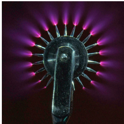
Corona discharge on a Wartenberg wheel.
