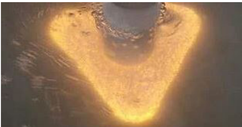
Plasma discharge around a component immersed in electrolyte.
