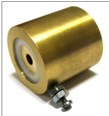
Faraday cup with an electron-suppressor plate in front.
