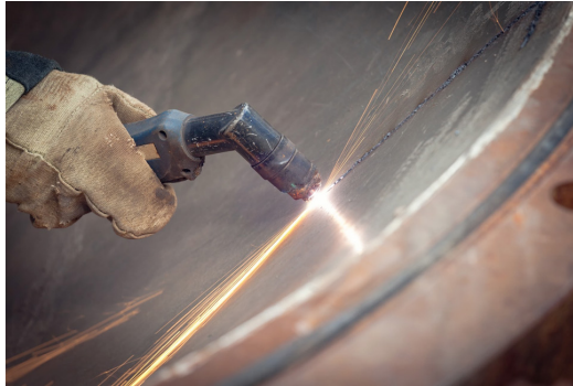
Handheld plasma arc cutting torch performing cutting operation.
