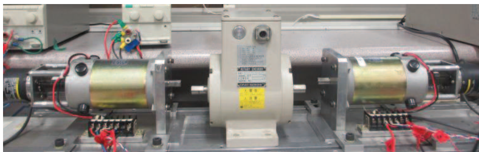
Figure 7. Photograph of three-mass resonance model.
