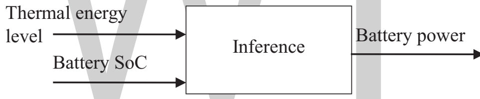
Figure 2. Fuzzy logic energy management inputs and output.
