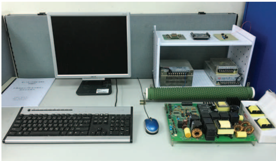
Figure 6. Photo and parameters of a PSPWM full-bridge power converter circuit. Transformer turns ratio n = 0.5 . V_i = 160 volt, V_0 = 50 volt, R = 6\Omega , C = 940\mu F L = 300\mu H , L_{lk} = 20\mu H C_A = C_B = C_C = C_D = 5nF , f_s = 50 kHz.
