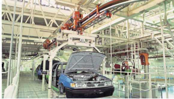
Overhead conveyor used in automobile assembly plant
