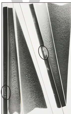
FIGURE 14: Porosity distribution in degassed A356 alloy castings obtained from the variable angle mold heated at 350°C.
