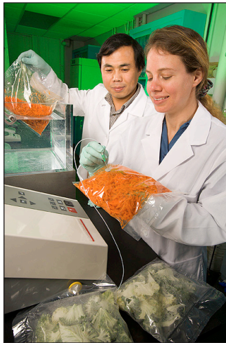
Testing modified atmosphere in a plastic bag of carrots.
