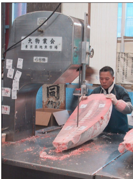
Cutting frozen tuna using a bandsaw in the Tsukiji fish market in Tokyo, Japan.
