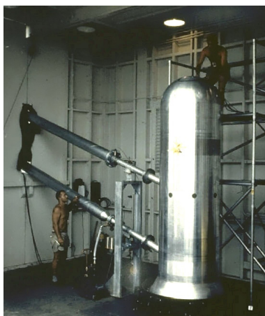
Bassoon, the prototype for a 9.3-megaton clean bomb or a 25-megaton dirty bomb. Dirty version shown here, before its 1956 test. The two attachments on the left are light pipes.
