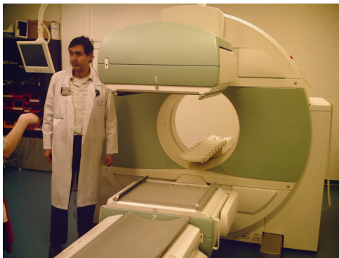
SPECT scanner, consisting of two gamma cameras.
