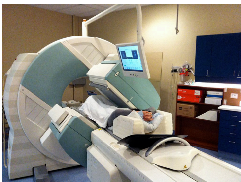
SPECT machine performing a total body bone scan. The patient lies on a table that slides through the machine, while a pair of gamma cameras rotates around her.
