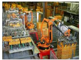
Automated palletizer of bread with industrial robots at a bakery in Germany.
