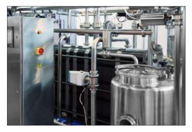
In ultrahigh temperature (UHT) pasteurisation milk and milk products are heated to at least 138°C for 2 sec and packaged aseptically. Pasteurised milk is not sterile it must be quickly cooled after pasteurisation to prevent multiplication of surviving bacteria. The effectiveness of pasteurisation is evaluated by phosphatase test which is alkaline phosphatase activity in milk.
