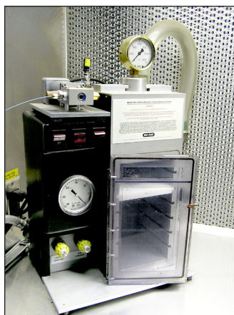
A gene gun uses biolistics to insert DNA into plant tissue.
