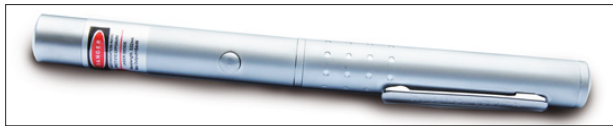
A green-emitting laser pointer, containing a tiny diode-pumped frequency-doubled solid-state laser. Red laser pointers are available in smaller sizes, because they do not need as large batteries.
