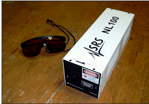
A 337nm wavelength and 170 \mu\text{J} pulse energy 20 Hz cartridge nitrogen laser.
