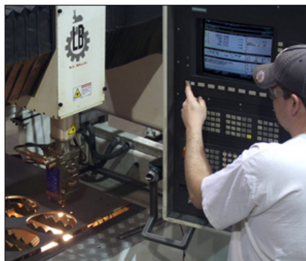
Industrial laser cutting of steel with cutting instructions programmed through the CNC interface.
