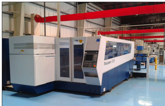
4000 watt CO 2 laser cutter.
