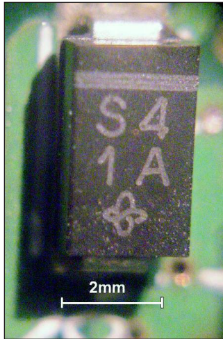
Laser marked electronic part.
