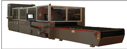
Dual-pallet flying optics laser.
