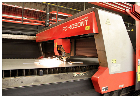
Flying optics laser head.
