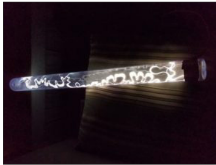
External triggering was used in this extremely fast discharge. Due to the very high speed, (3.5 microseconds), the current is not only unable to fully heat the xenon and fill the tube, but is still in direct contact with the glass.
