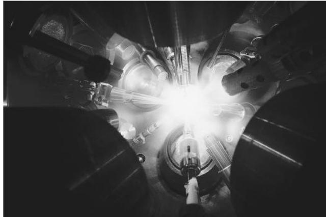
Lasers focus on a small pellet of fuel in attempt to create a nuclear fusion reaction (the combination of two nuclei to produce another nucleus) for the purpose of producing energy.
