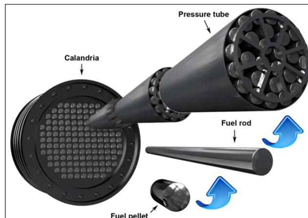
These pellets contain the radiation. They form the first layer of containment. The pellets are enclosed in rods, which form the second layer of containment. CANDU fuel rods are made of zircaloy, a metal alloy extremely resistant to heat and corrosion.
