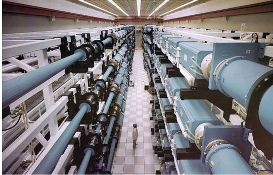
Currently, high powered Nd:glass lasers as large as a football field are used for inertial confinement fusion, nuclear weapons research, and other high energy density physics experiments.
