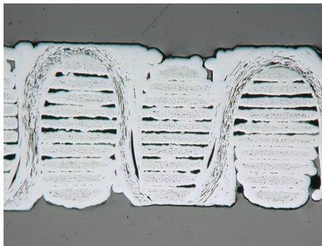
Micrograph of a SiC/SiC ceramic composite with a woven three-dimensional fibre structure.
