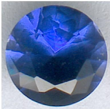
Synthetic sapphire - single-crystal aluminum oxide
