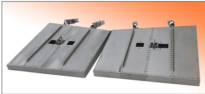
Pair of steering flaps for the NASA-space vehicle X-38. Size: 1.5×1.5×0.15 m, mass: 68 kg each, various components are mounted using more than 400 CVI-C/SiC screws and nuts.
