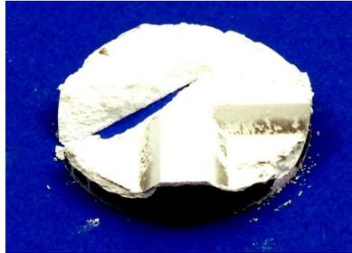
A piece (formed with M KMS-96 alumina powder) has been broken after mold ejection.
