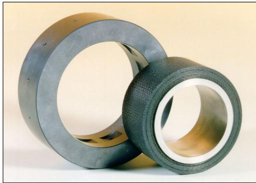
Components for a ceramic slide bearing; the picture shows a sintered SiC-bearing for a hydrostatic slide bearing and a CVI-SiC/SiC-shaft sleeve shrink-fitted on metal, a system tested with liquid oxygen as lubricant.
