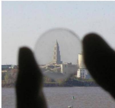
Transparent spinel ( $\text{MgAl}_2\text{O}_4$ ) ceramic is used traditionally for applications such as high-energy laser windows because of its excellent transmission in visible wavelengths and mid-wavelength infrared (0.2-5.0 $\mu\text{m}$ ) when combined with selected materials.
