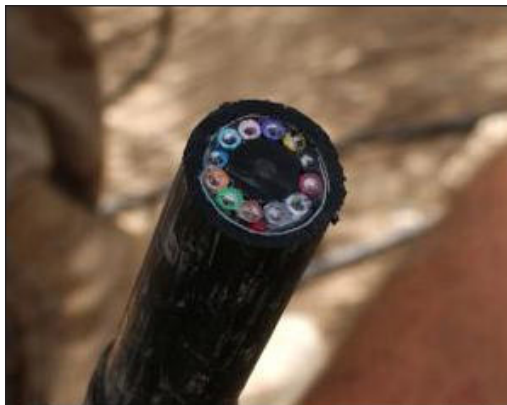
A section of 144-strand fiber-optic cable. Each strand is made of optically pure glass and is thinner than a human hair.
