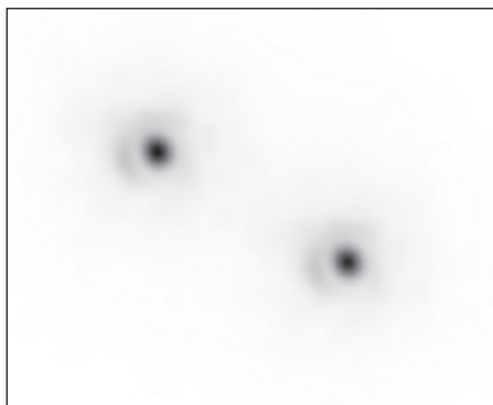
The Airy disk around each of the stars from the 2.56 m telescope aperture can be seen in this lucky image of the binary star zeta Boötis.
