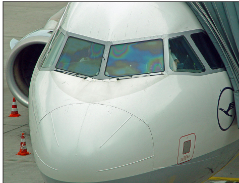
Thin film interference caused by ITO defrosting coating on an Airbus cockpit window. The film thickness is intentionally non-uniform to provide even heating at different distances from the electrodes.
