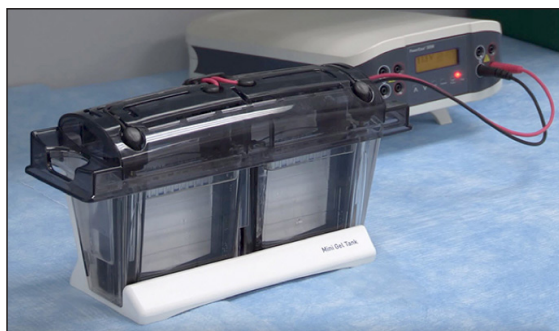
Polyacrylamide gel electrophoresis in progress.
