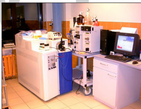
Quadrupole Time-of-Flight tandem Mass Spectrometer (Q-TOF)
