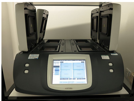
A thermal cycler for PCR.
