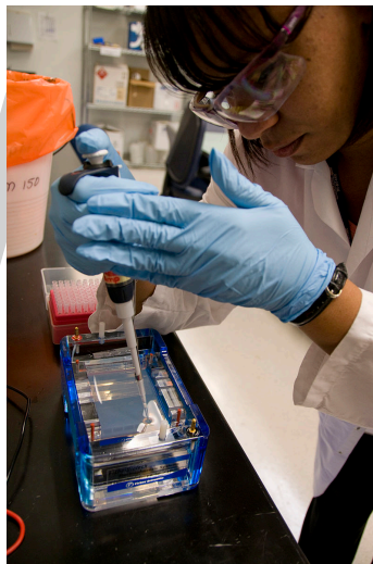
FDA microbiologist prepares DNA samples for gel electrophoresis analysis.
