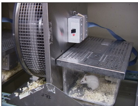
Mouse from the Garland selection experiment with attached running wheel and its rotation counter.
