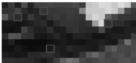
Fig. The Graphic Shows how Information can be Hidden in a Picture. The Encryption Software Includes Information by Altering the Information of Certain Pixels. If the Picture is Sufficiently Large, Changes can Hardly be Recognised without Having Access to the Original, as well as the Modified, Picture. Using this Technology, Offenders Can Hide the Fact that they are Exchanging Additional Information.
