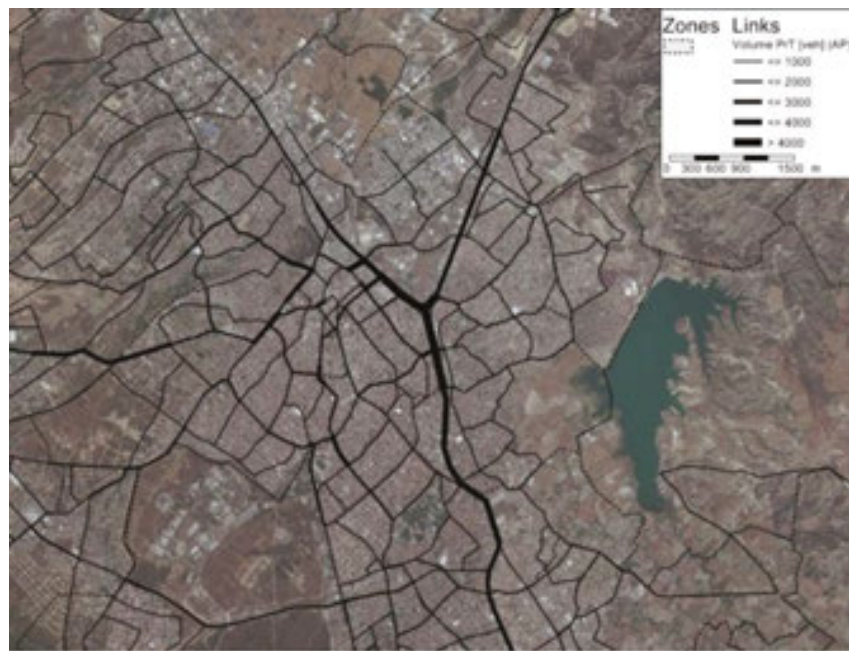
Figure 5. Traffic volumes on the road network for 2010.
