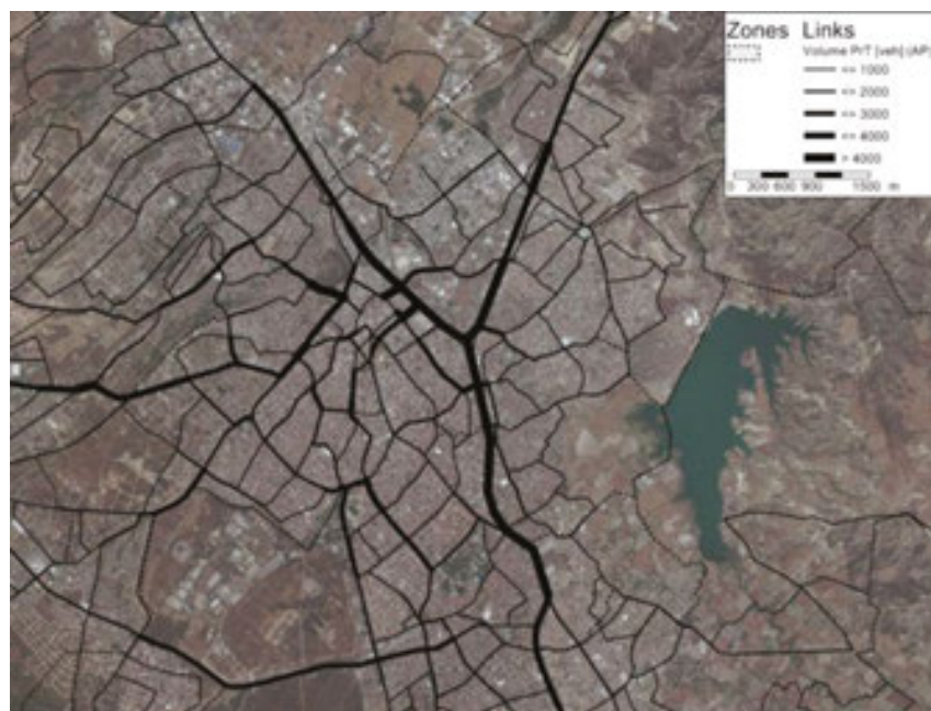
Figure 6. Traffic volumes on the road network for 2030.
