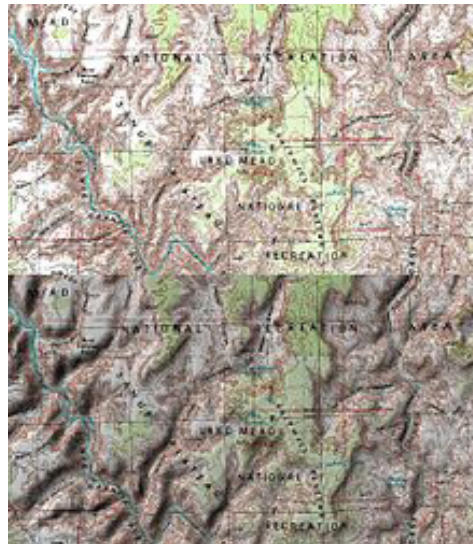
Top: map of Lake Mead area Bottom: the same map with sun shading
