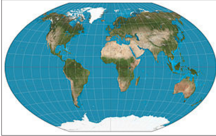
A world map on the Winkel tripel projection, a low-error map projection.
