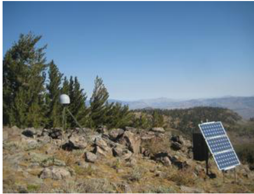
High precision GPS station in the Sierra Nevada region of in the Plate Boundary Observatory (station P149).
