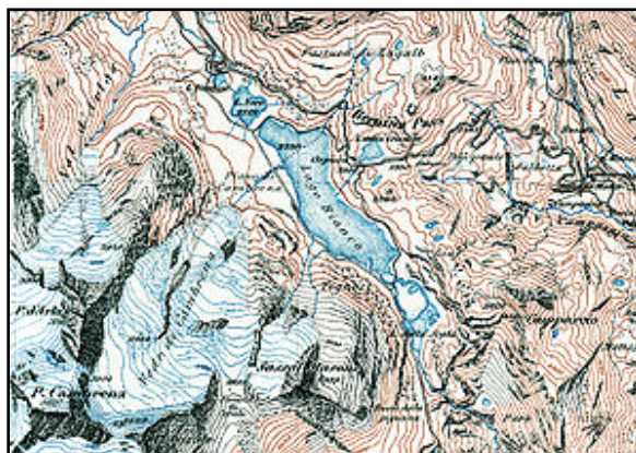
Siegfried map of Bernina Pass with black, blue and brown contour lines at 30-meter intervals.
