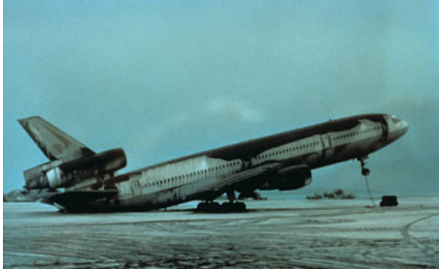
Mount Pinatubo, Philippines: View of World Airways DC-10 airplane setting on its tail because of weight of June 15, 1991 ash. Cubi Point Naval Air Station.
