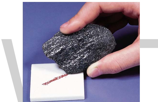
The streak of this dark gray mineral (hematite), obtained by rubbing it on the white streak plate is reddish brown.
