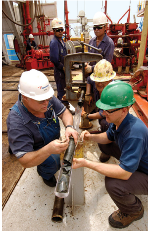
Crew members aboard a drilling ship inspecting a rock core during a scientific expedition that succeeded for the first time in drilling through the upper oceanic crust.
