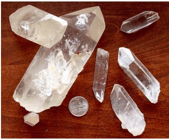
Crystal of quartz. Sides form a hexagonal prism that is capped with pyramid-like faces. Note the fine grooves on some crystal faces.
