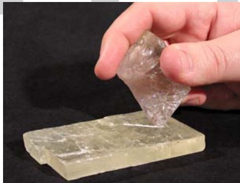
Testing mineral hardness. The harder mineral (quartz) scratches the softer one (calcite)
