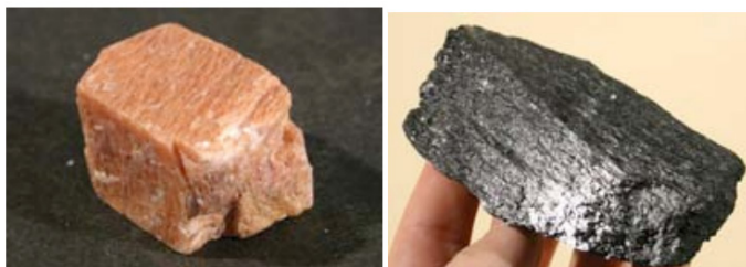
Two directions of cleavage: A. Cleavages in potassium feldspar intersect at 90^\circ ; B. Prismatic cleavages in hornblende intersect at 56^\circ and 124^\circ .
