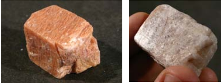
The thin veinlets seen in some potassium feldspars (left) should not be confused with striations in plagioclase (right). Striations are visible on the upper surface of this sample of plagioclase.
