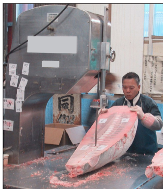
Cutting frozen tuna using a bandsaw in the Tsukiji fish market in Tokyo, Japan.
