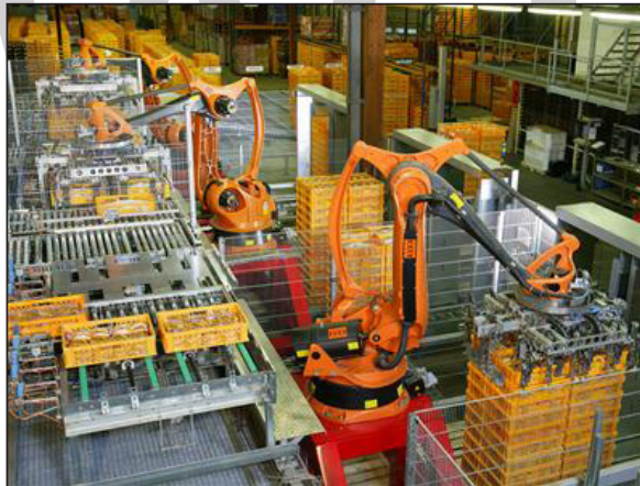
Automated palletizer of bread with industrial robots at a bakery.
