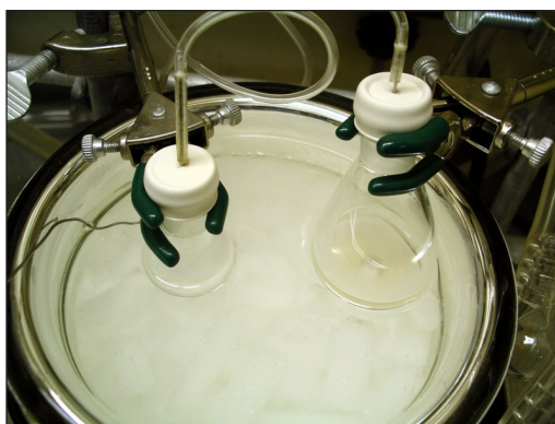
A typical experimental setup for an aldol reaction. Both flasks are submerged in a dry ice/acetone cooling bath ( -78\text{ }^{\circ}\text{C} ) the temperature of which is being monitored by a thermocouple (the wire on the left).
