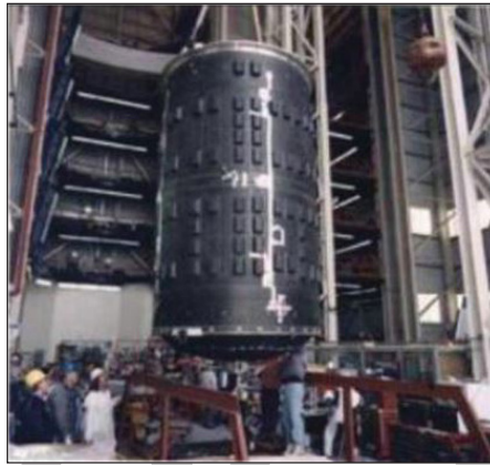
DC-XA composite LH 2 cryotank.
