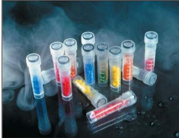
Cryotubes used to store strains of bacteria at low temperature. Bacteria are placed in little holes in the beads inside the tubes and then stored in liquid nitrogen.
