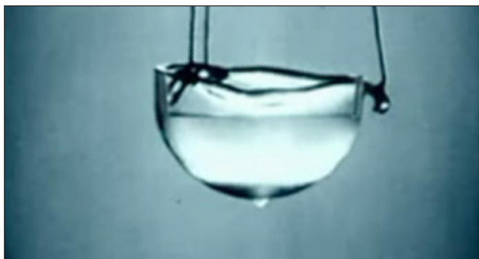
When cooled below the Lambda point ( 2.17\text{ K} or -270.98\text{ }^{\circ}\text{C} at 1\text{ atm} ), liquid helium exhibits properties of superfluidity.
