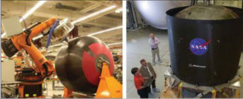
2.4 m diameter tank, a robotic arm applies composite laminate.
