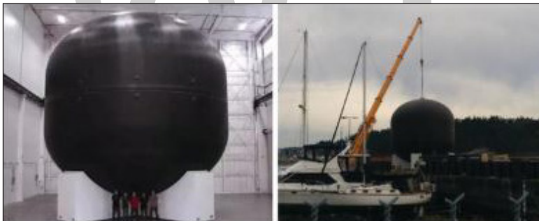
The 12-m diameter composite lox tank of space X.
