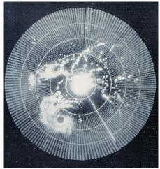
Brightness can indicate reflectivity as in this 1960 weather radar image (of Hurricane Abby). The radar's frequency, pulse form, and antenna largely determine what it can observe.
