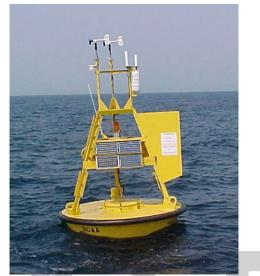
Weather buoy operated by the NOAA National Data Buoy Center.
