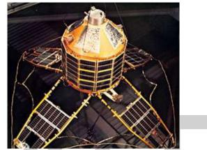
The British Ariel 4 (U.K. 4), shown suspended with its solar panels deployed in flight configuration. It was launched Dec. 11, 1971, by NASA (National Aeronautics and Space Administration) and surveyed the ionosphere and certain radio signals.
