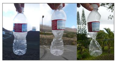
This plastic bottle was sealed at approximately 14,000 feet (4,300 m) altitude, and was crushed by the increase in atmospheric pressure, recorded at 9,000 feet (2,700 m) and 1,000 feet (300 m), as it was brought down towards sea level.
