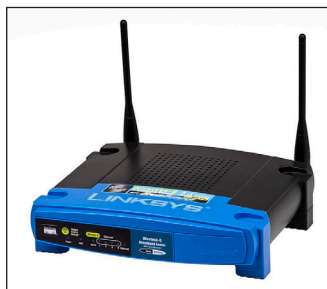
In a wireless computer network, wireless routers like this contain a 2.4 GHz transmitter that sends and receives network packets for computers on the local area network.
