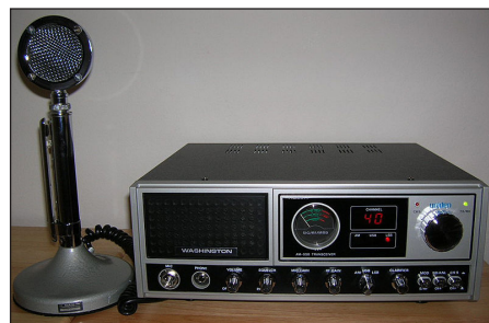
A CB radio transceiver, a two way radio transmitting on 27 MHz with a power of 4 W, that can be operated without a license.
