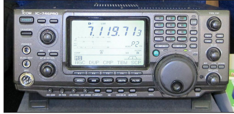
Modern amateur radio transceiver, the ICOM IC-746PRO. It can transmit on the amateur bands from 1.8 MHz to 144 MHz with an output power of 100 W.
