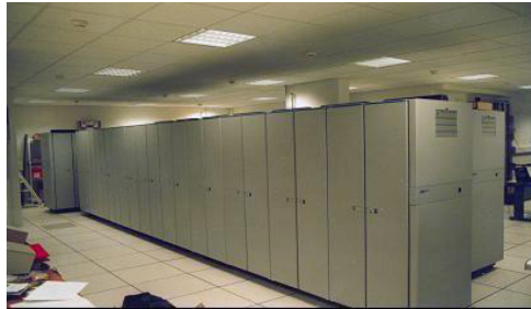
A digital exchange (Nortel DMS-100) used by an operator to offer local and long distance services in France. Each switch typically serves 10,000–100,000+ subscribers depending on the geographic area.
