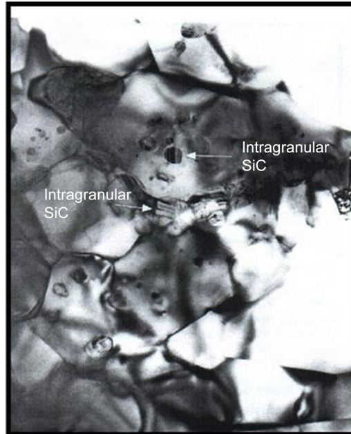
Actual microstructure of a SiC-Si 3 N 4 nanocomposite.
