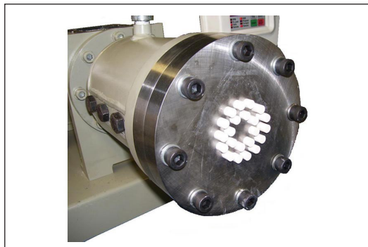
A multiple-hole plate is commonly used in pelletizing.
