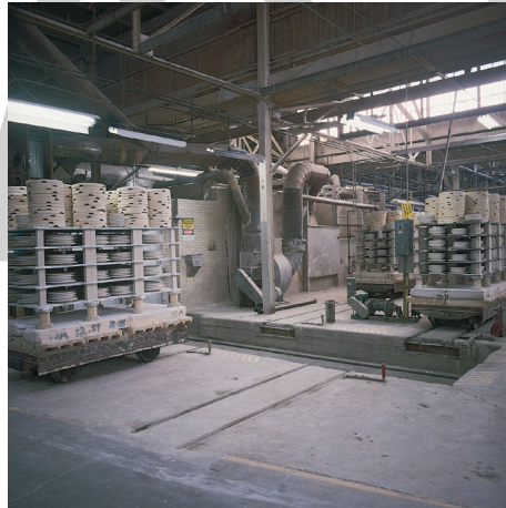
Unfired whiteware stacked on kiln carts prior to firing.
