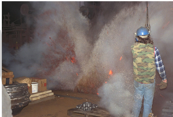
A retained fragment of sand core in an industrial impellor explodes during quenching.
