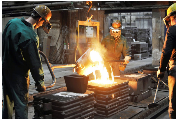
Steel castings are solid metal objects produced by filling the void within a mold with liquid steel.
