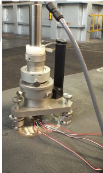
The need of positioning the drill cutter with absolute precision and the need of executing the drilling at controlled depth requires the use of specific drilling equipment.
