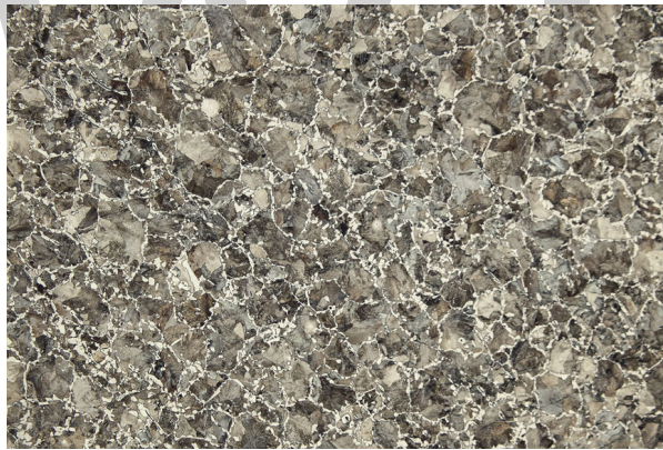
Heat treatment like annealing creates rounder grains that create a more ductile metal.
