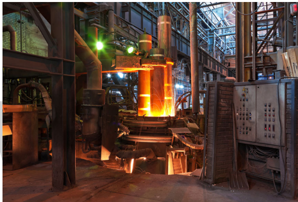
The electric arc furnace melts batches of metal using graphite electrodes; the charge passes directly between the electrodes, exposing it to thermal energy.
