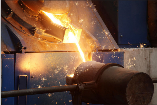
An induction furnace is an electrical furnace where heat energy is transferred by induction, and can operate with minimal melt loss.
