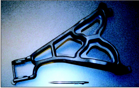
Austempered ductile iron suspension arm for a Ford Mustang Cobra.
