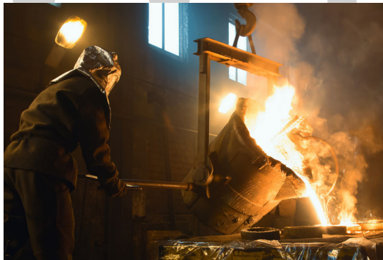
During heat analysis, a sample of liquid cast steel is ladled from the furnace, allowed to solidify, and then analyzed for chemical composition using spectrochemical analysis.
