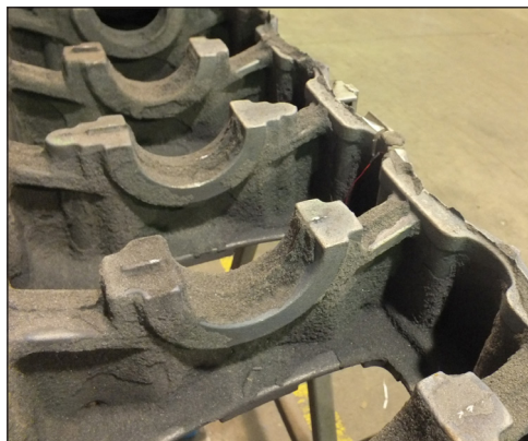
The casting of an engine block: with its complex geometry and its alternation of walls with different thickness, it is a typical applicative example for the cutting technique.
