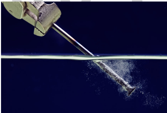
Quenching metals helps to harden them using thermal shock.
