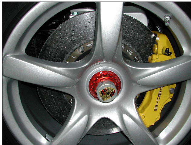
The Porsche Carrera GT's carbon-ceramic (silicon carbide) disc brake.
