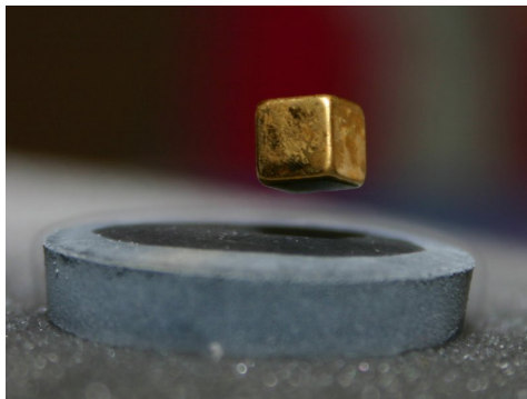
The Meissner effect demonstrated by levitating a magnet above a cuprate superconductor, which is cooled by liquid nitrogen.
