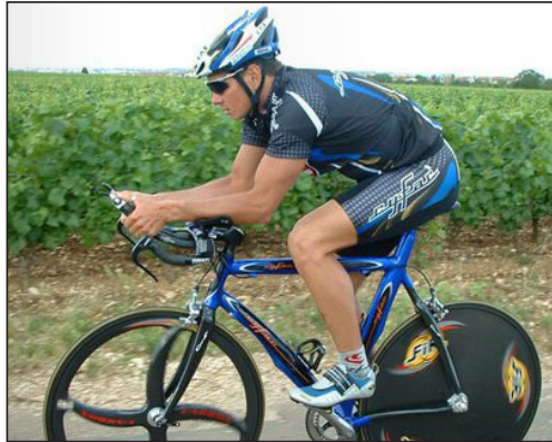
A time-trial carbon fibre composite bicycle with aerodynamic wheels and aero bars.
