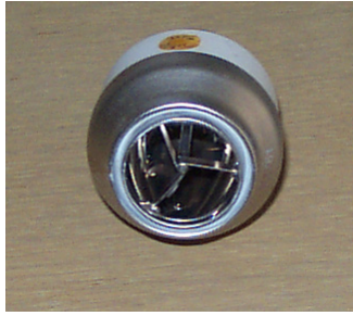
Cermax xenon arc lamp with synthetic sapphire output window.
