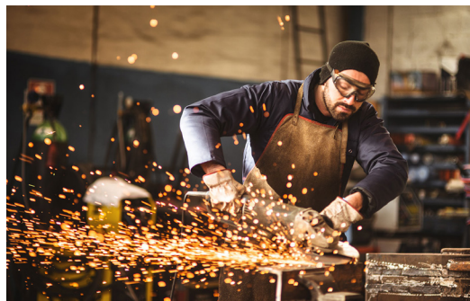
Angle grinder Worker using an angle grinder to smooth a piece of metal.
