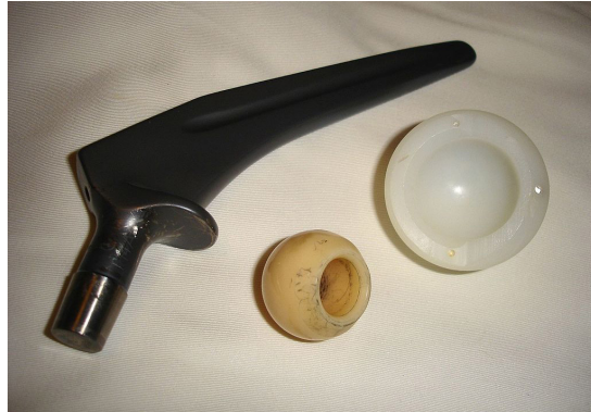
A titanium hip prosthesis, with a ceramic head and polyethylene acetabular cup.
