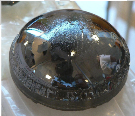
Silicon carbide single crystal.
