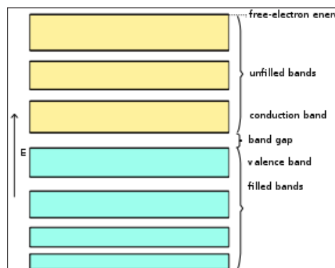
Band structure of a semiconductor showing a full valence band and an empty conduction band.
