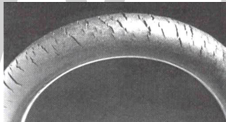
Ozone cracking in Natural rubber tubing
